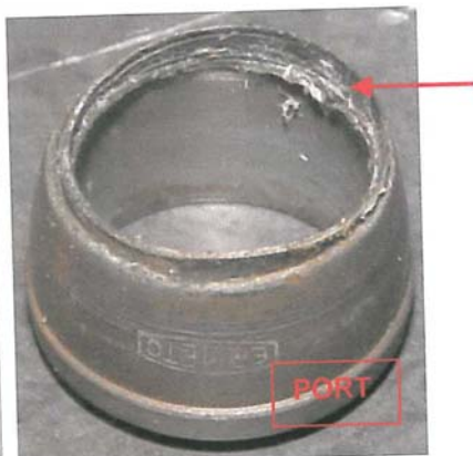
Photo 9: Port side ferrell showing metal deposits - red arrow (digital)
