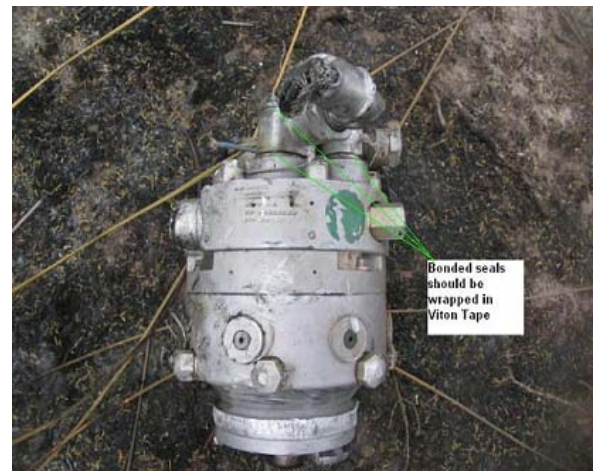
Figure 6, shows hydraulic pump.
