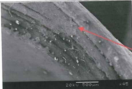
Photo 10: Port side ferrell, showing pipeline deposit (x45, SEM)
