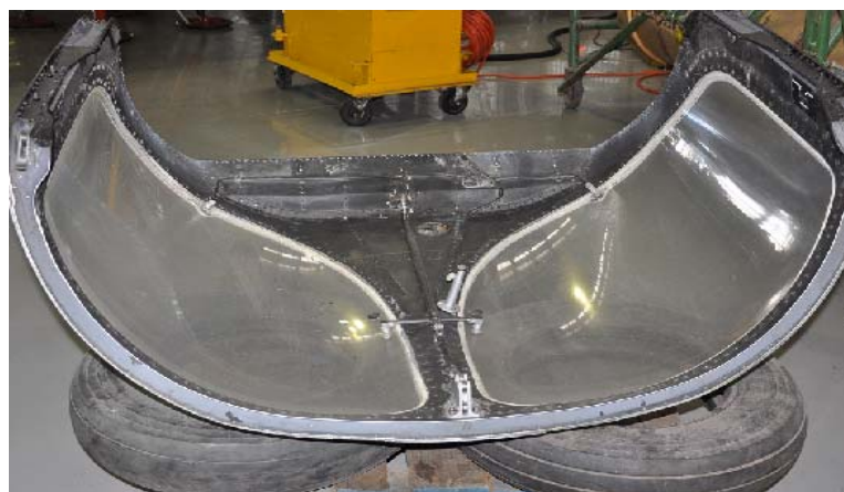
Figure 41, shows type of canopy installed on the lightning aircraft
