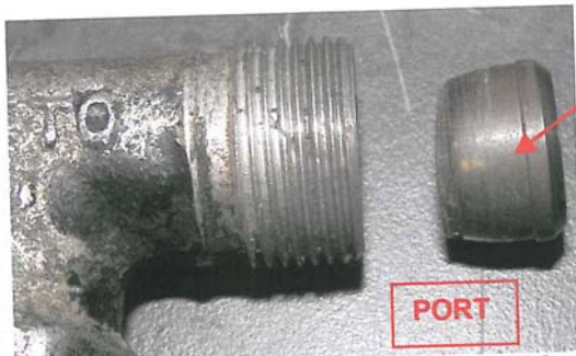
Photo 8: Port side pipeline ferrell removed from position, as found (digital)
