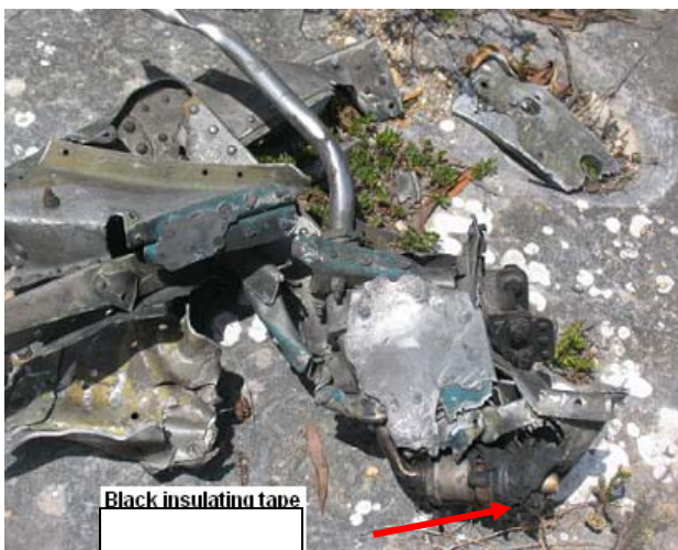
Figure 7 & 8, shows black rubber material wrapped around connecting couplings.
