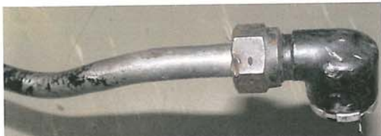
Photo 5: Primary cartridge end of pipeline showing fractured breech (digital)
