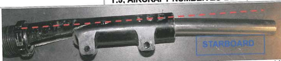
Photo 20: Starboard high velocity canopy jack showing bending damages (digital)
