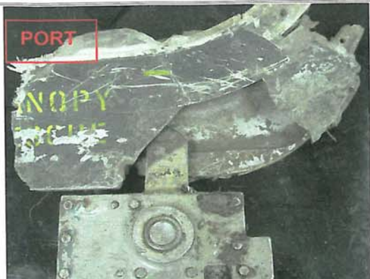
Photo 17: Port side, main canopy hook in canopy frame position, showing extensive damages (digital)
