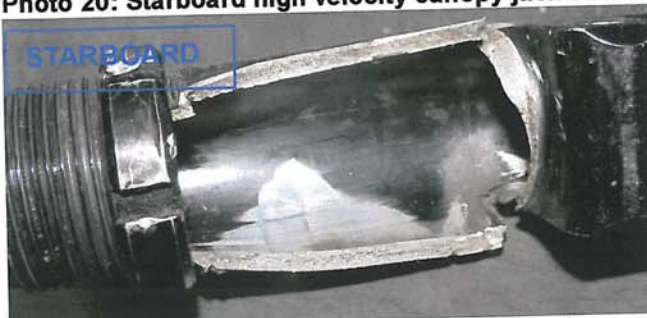
Photo 21: Starboard canopy jack sleeve showing explosion damages (digital)
