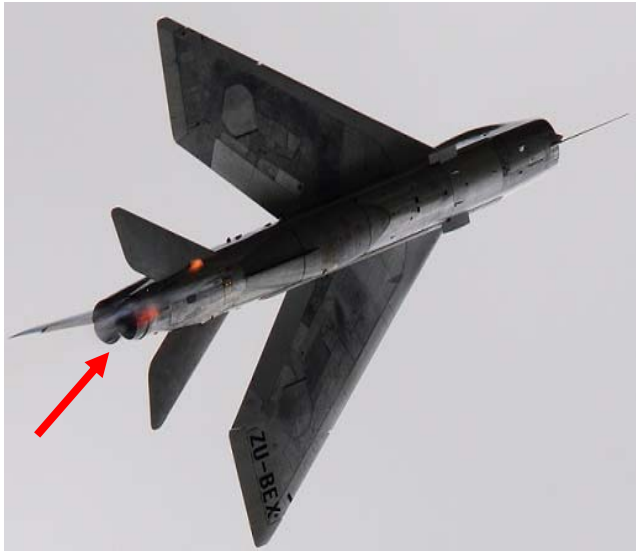
Figure 34 & 35, show proof of atomised fluid from the tail section of EE Lightning.
