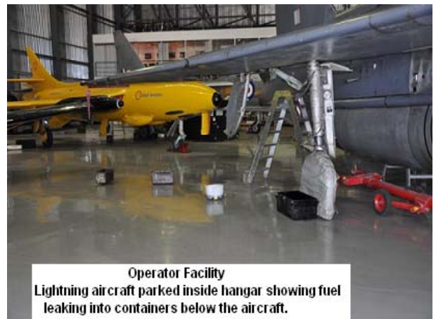
Figure 33, show fuel leaking from another EE Lightning at AMO.
