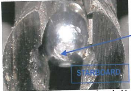
Photo 15: Piston crown, starboard side by-pass valve piston, showing indentation marks (digital)
