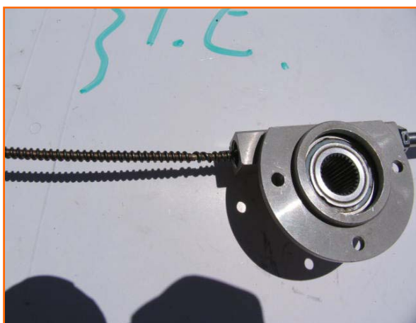
A view of the steering control box with the damaged control cable inserted and the outer cable casing removed to expose the damage to the cable.
