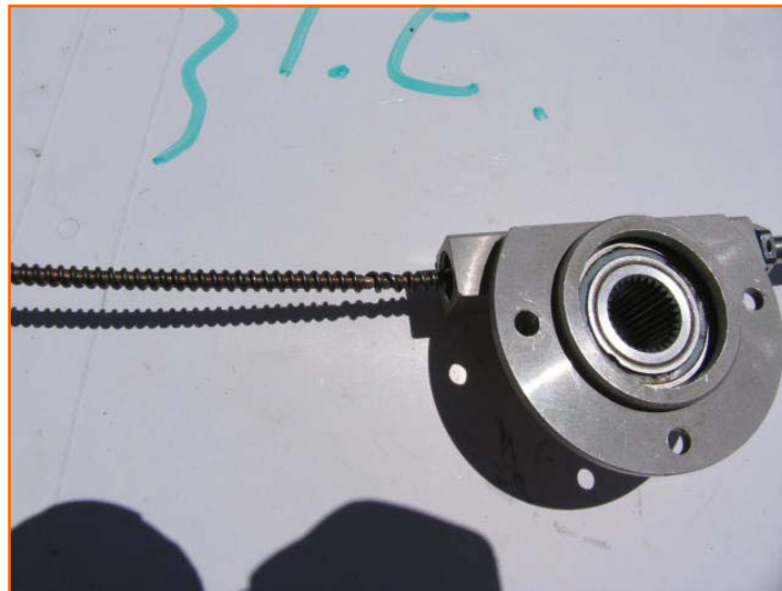
Fig 4: A view of the steering control box with the damaged control cable inserted and the outer cable casing removed to expose the damage to the cable.
