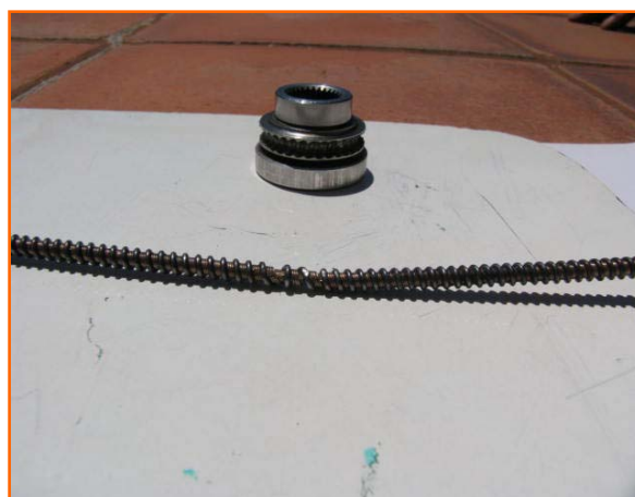
A view of the gear inside the steering control box, showing the damaged Control cable (Stretch & Kink) next to it
