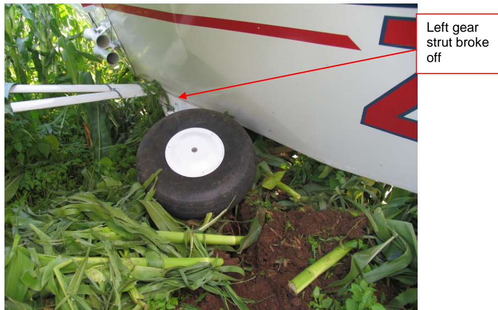
Figure 3. The damaged left main gear.
