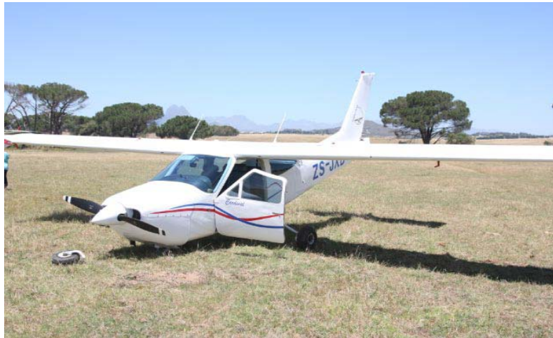
Figure1: Showing the broken nose wheel
