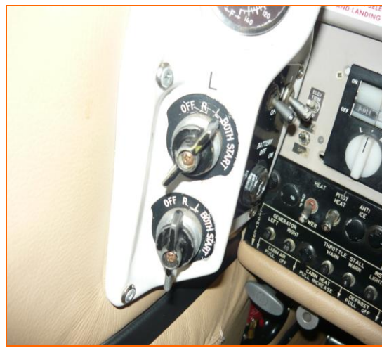
Figure 7: The magneto switches on the wreckage: The left-hand engine was selected on the left magneto and the right-hand engine was selected on the right magneto.
