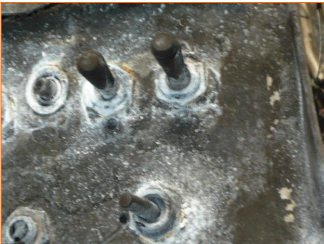
Figure 7: The fuel booster pumps on the wreckage were in the High position.
