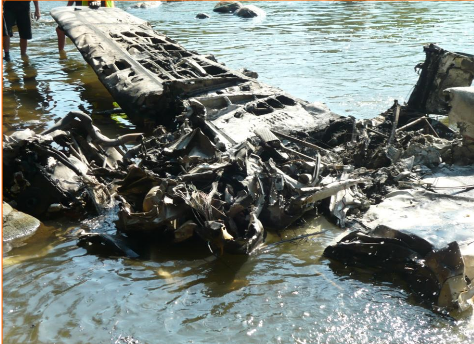
Figure 6: The wreckage was destroyed by the impact damage and the ensuing fire after the impact.
