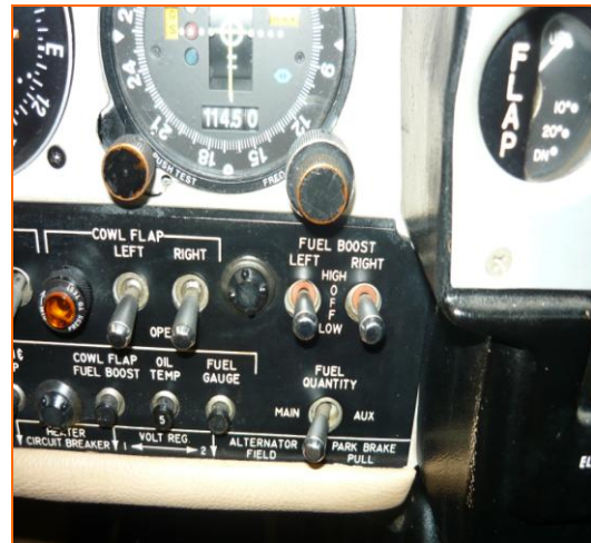
Figure 7: The fuel booster pumps on the wreckage were in the High position.
