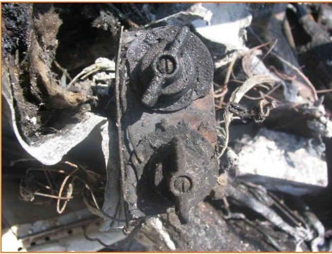
Figure 7: The magneto switches on the wreckage: The left-hand engine was selected on the left magneto and the right-hand engine was selected on the right magneto.
