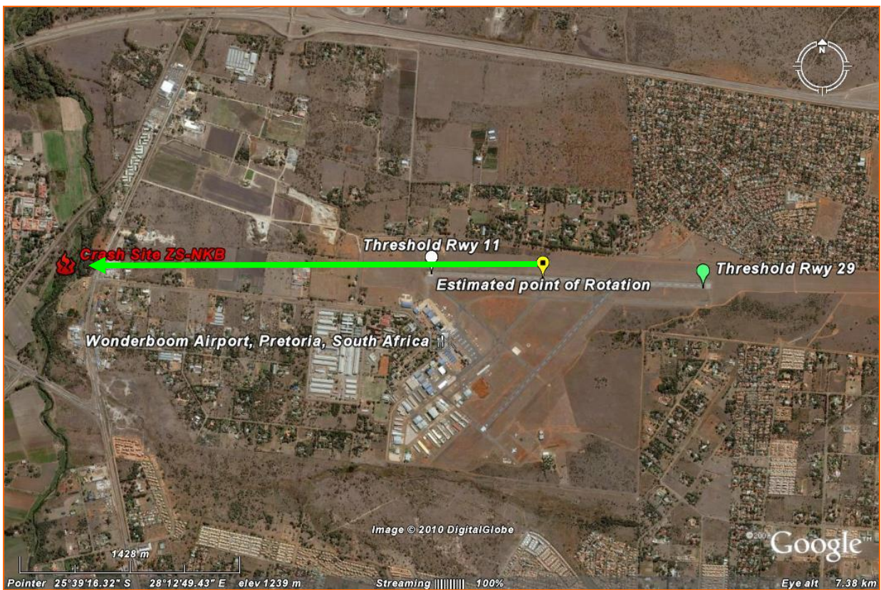
Figure 4: Aerial view of the flight path followed from takeoff on Rwy 29 to the accident site
