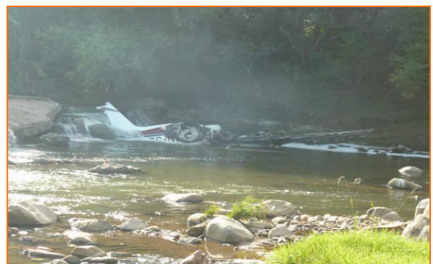
Figure 3: View of the wreckage in the river with the empennage against a retainer wall in the river.
