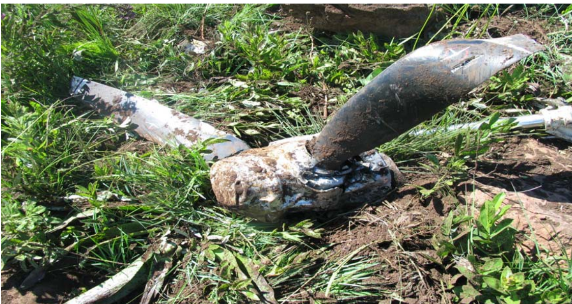
Figure 4: The damaged propeller
