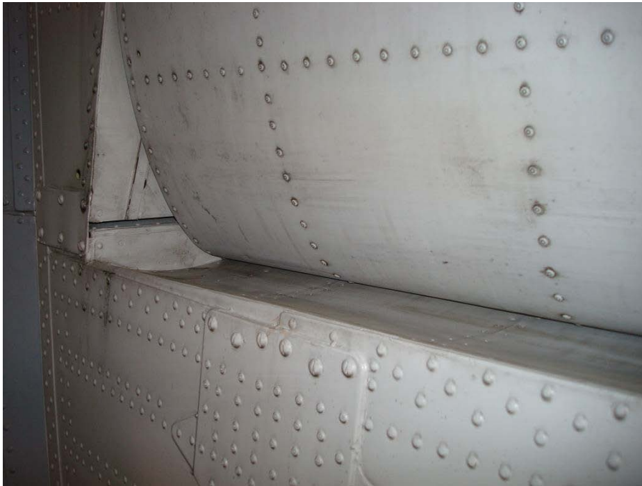
Fig. 20. Elevator clearance at position 1.
