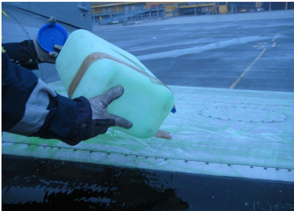
Fig. 11. Application of Type IV fluid in connection with the tests.
