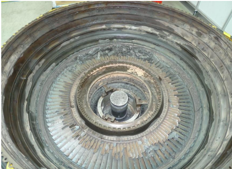
Fig. 40. LPT guide vanes and turbine blades stage two. Photo: SHK.
