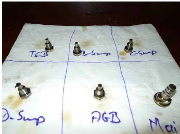
Fig. 41. The oil system's chip plugs; only the D sump (LPT) plug had traces of magnetic material. The number of chips was normal for the operating time. Photo: SHK.
