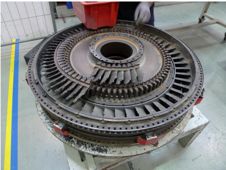
Fig. 39. HPT stage two. Photo: SHK.
