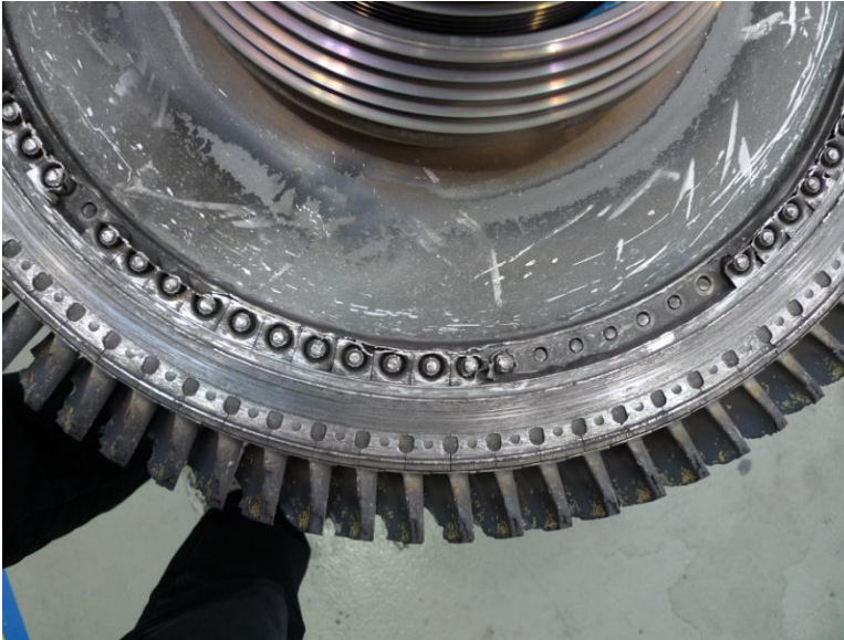
Fig. 38. HPT disc and turbine stage one with Diffuser Front Seal. Photo: SHK.
