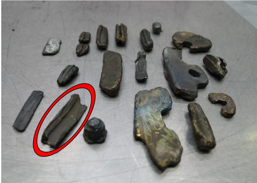
Fig. 44. Fragments analysed by Volvo Aero Corporation. The piece marked in red is a piece of the edge of the diffuser aft air seal. Photo: SHK.
