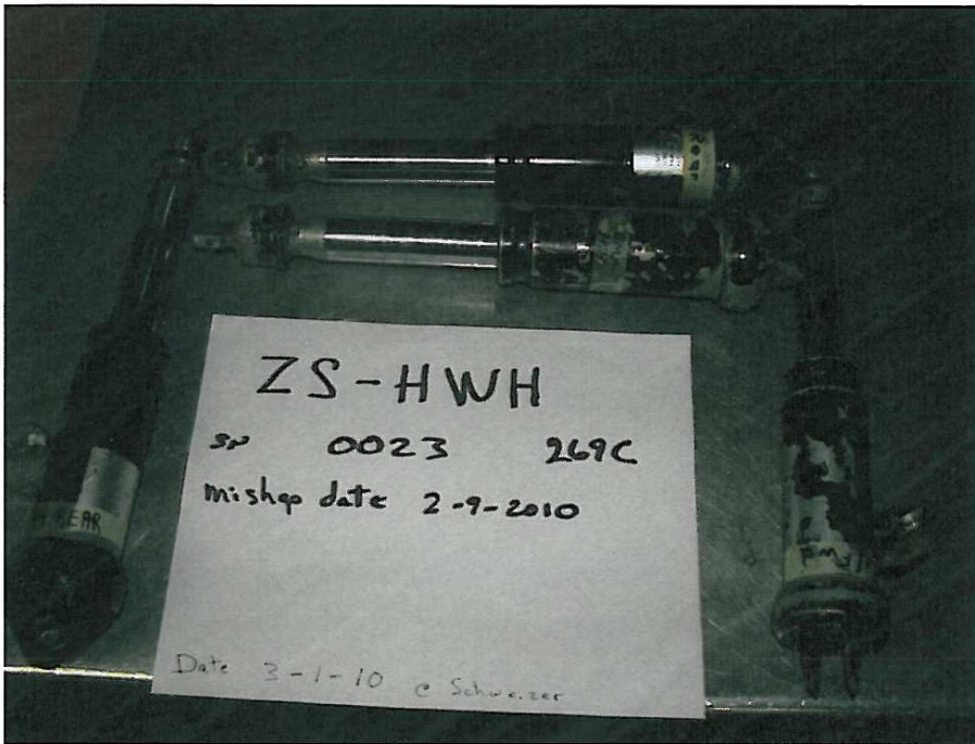
Fig 2 Dampers as received at Schweizer for load stroke testing
