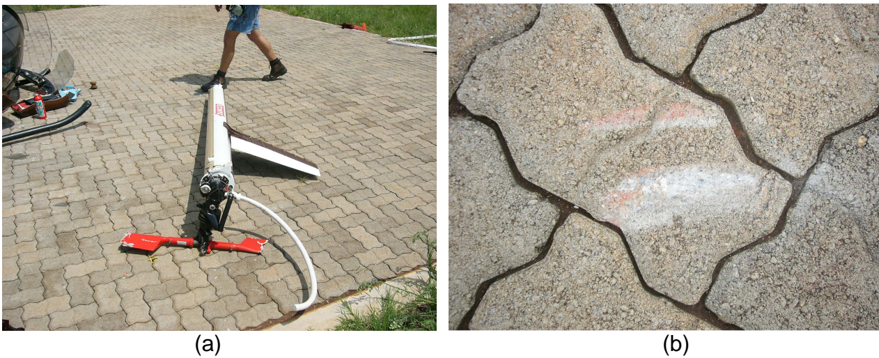
Figure 3 Damage to the tail rotor blades (a) and contact marks (b) with the landing surface
