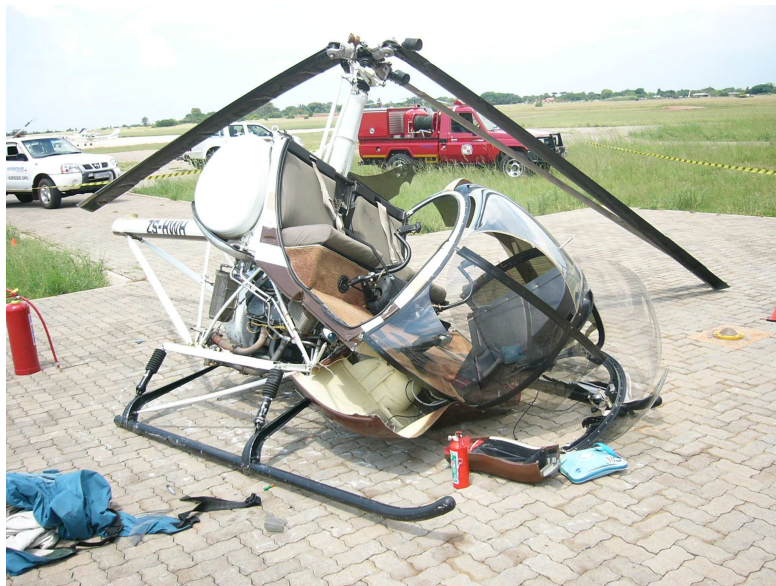
Figure 1 Damage caused to the fuselage of the helicopter
