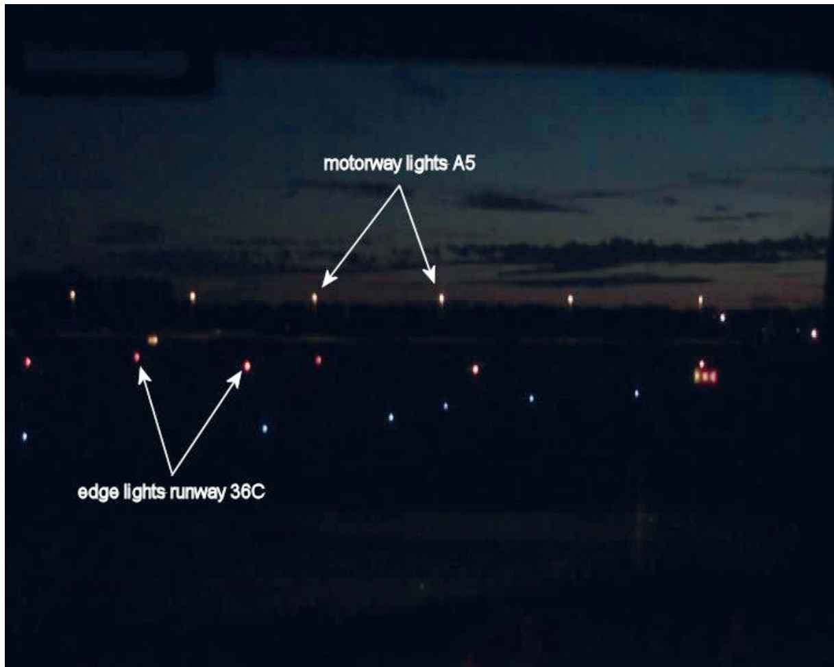
Figure 10: Patterns of the edge lights on runway 36C and the lights of the A5 motorway
