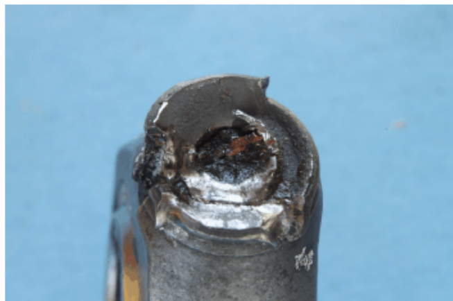
Figure 3. The ball-joint end fracture surface showing only ductile overload features.
