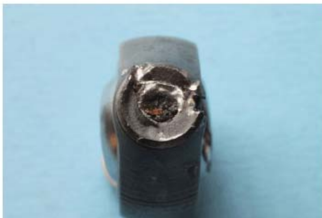
Figure 2. The ball-joint end fracture surface showing only ductile overload features.
