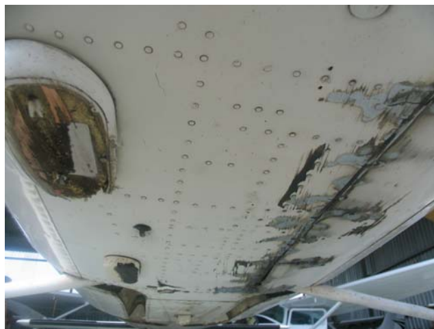
Figure 2: Damage to the belly and antenna.
