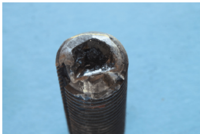
Figure 4. The threaded end of the fracture showing severe battering.
