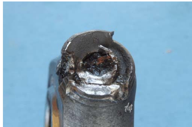
Figure 5. Another view of the ball-joint end fracture surface.
