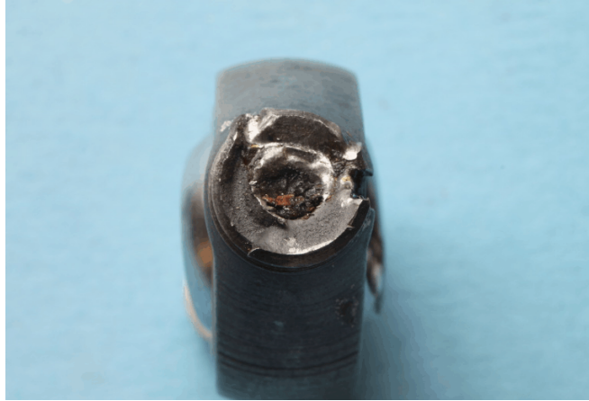
Figure 4. The ball-joint end fracture surface showing ductile overload.
