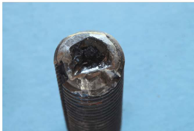
Figure 6. The threaded end of the fracture showing severe battering.
