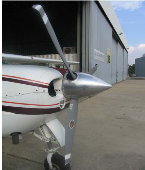
Figure 1. The bent propeller tips.
