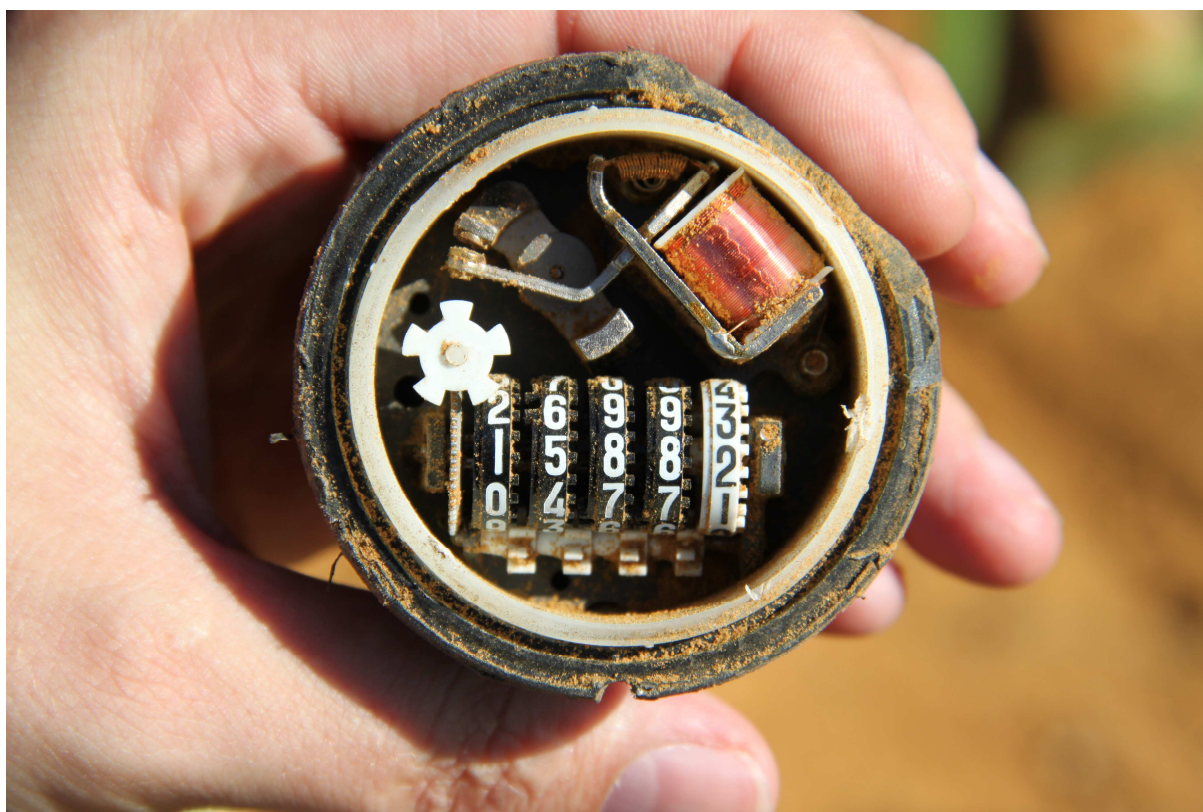
Photo 2: Hobbs meter reading as found on accident site
