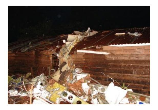
As shown in the wreckage photo above, the aircraft was completely destroyed on impact to the ground before the wreckage and debris scattered, much of which were restrained by the wooden house structure. There were some debris on the iron sheet roof of the house while some were found scattered within the compound within a radius distance of 40m from the point of impact with the ground.
