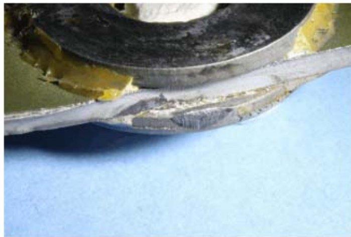
Figure 4. Thumb-nail feature, indicating initiation site, concealed beneath reinforcing washer.
