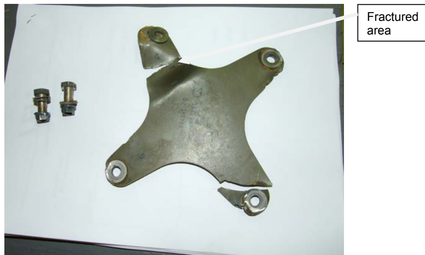
Figure 2: Fractured forward flex plate
