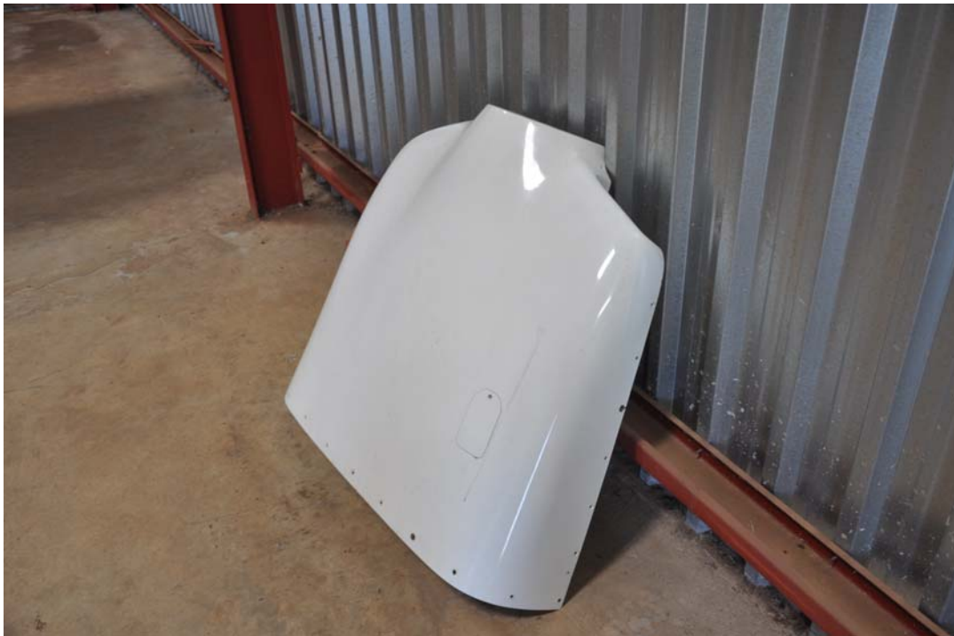
Figure 3. The engine cowling, which was removed before the ground-runs.
