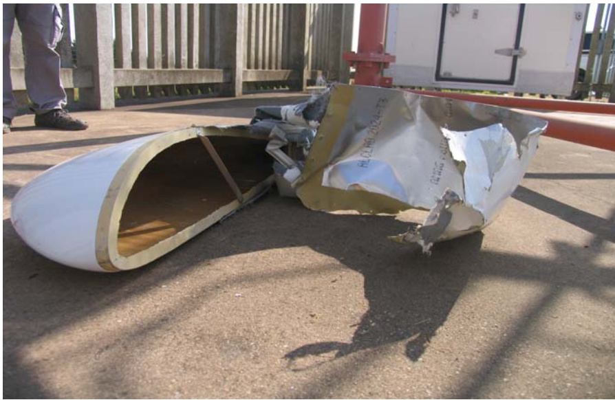
Figure 3. The right wingtip and part of the outer wing.
