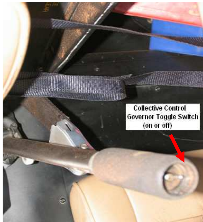
Figure 5. The position of the governor toggle switch.
