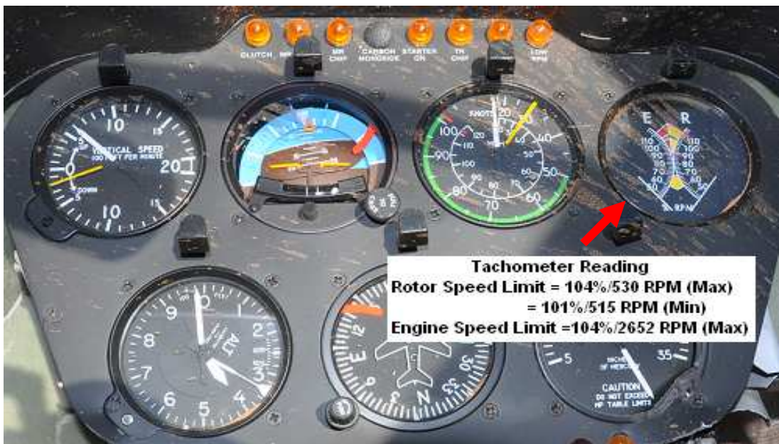
Figure 4. The instrument panel of ZS-RRM, showing the tachometer measuring rotor and engine RPM.
