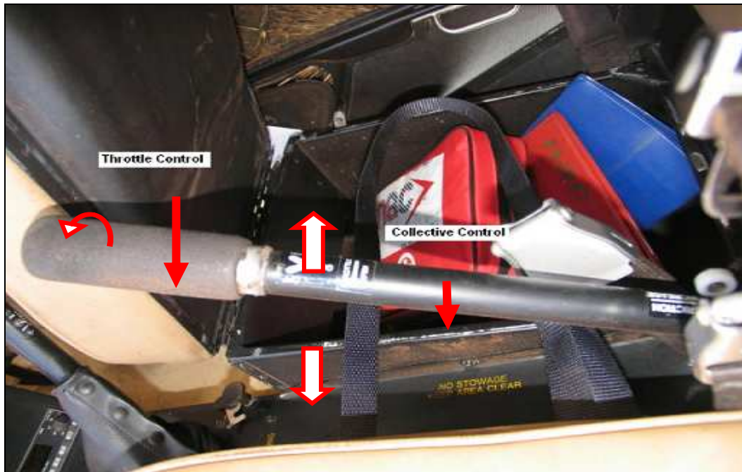
Figure 3. The collective pitch lever and throttle control lever.
