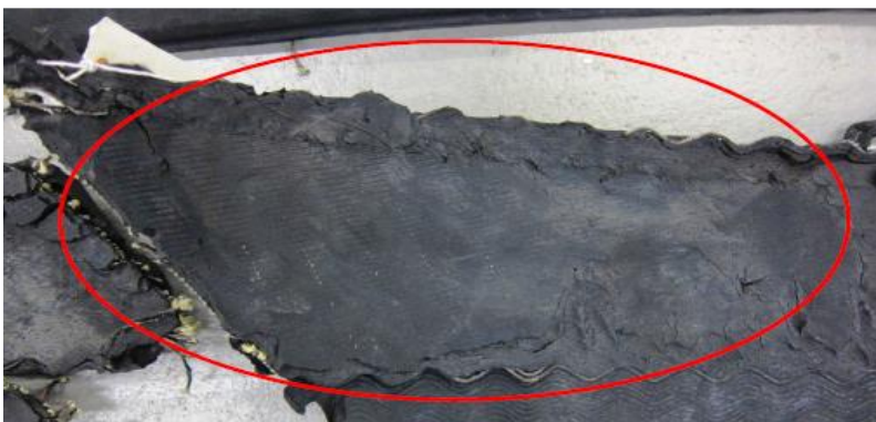
Figure 8. Heat buildup indications.
