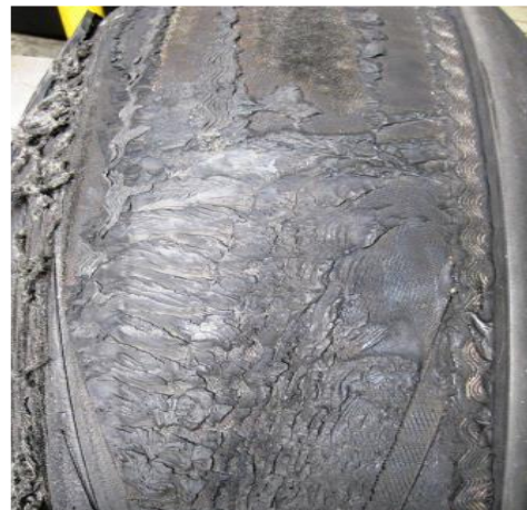
Figure 5. Separation surface (detail).
