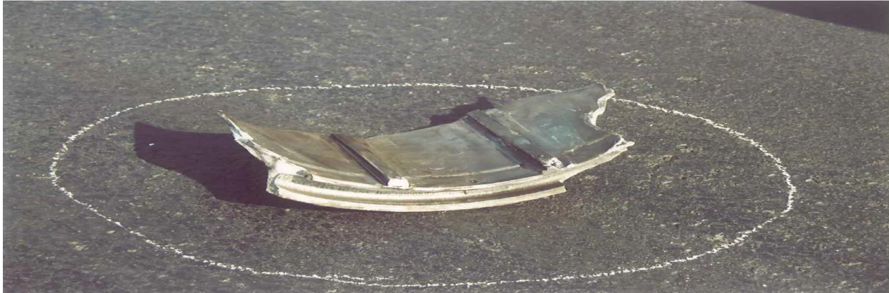
Figure 13. The Piece of the Wheel Rim, which was the cause of the Nose Landing Gear Collapse.
