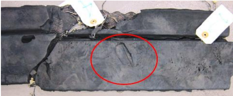
Figure 6. Indentation on the center rib.
