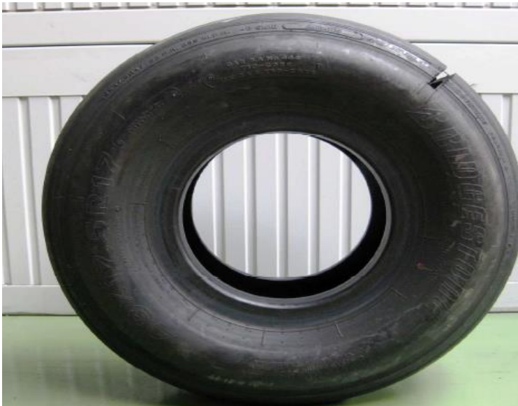
Figure 2. The failed tire outboard sidewall.
