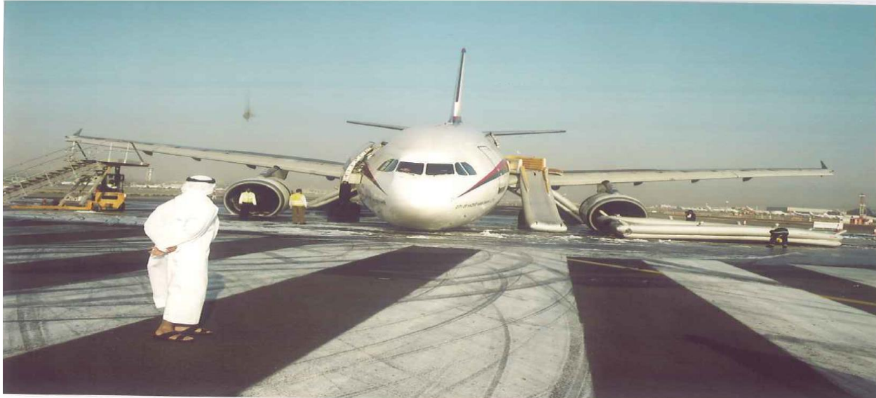
Figure 12. The A-310, following the Collapse of the Nose Landing Gear, after hitting an FOD on the take-off runway.
