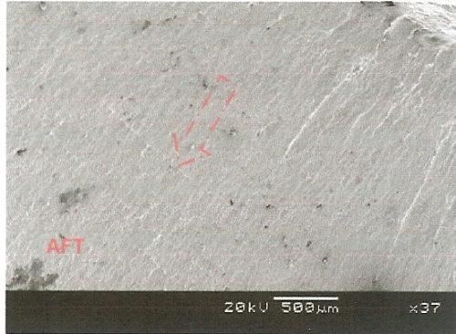
Photo 8: Fatigue beach marks on fracture surface, AFT end (x37, SEM)
