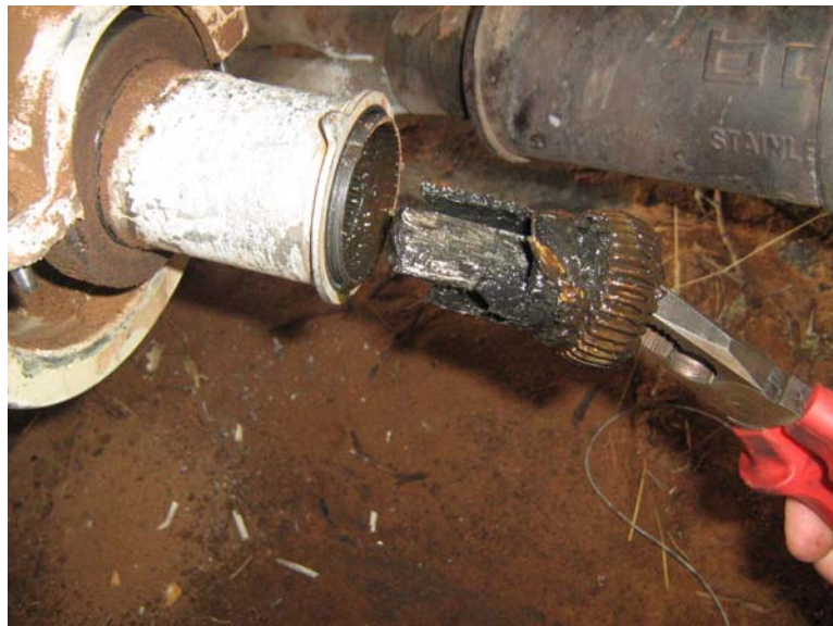
Figure 3. A view of the failed driveshaft being removed from the drive pulley assembly.
