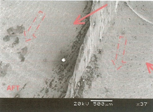
Photo 7: Fatigue beach marks on fracture surface, AFT end (x37, SEM)
