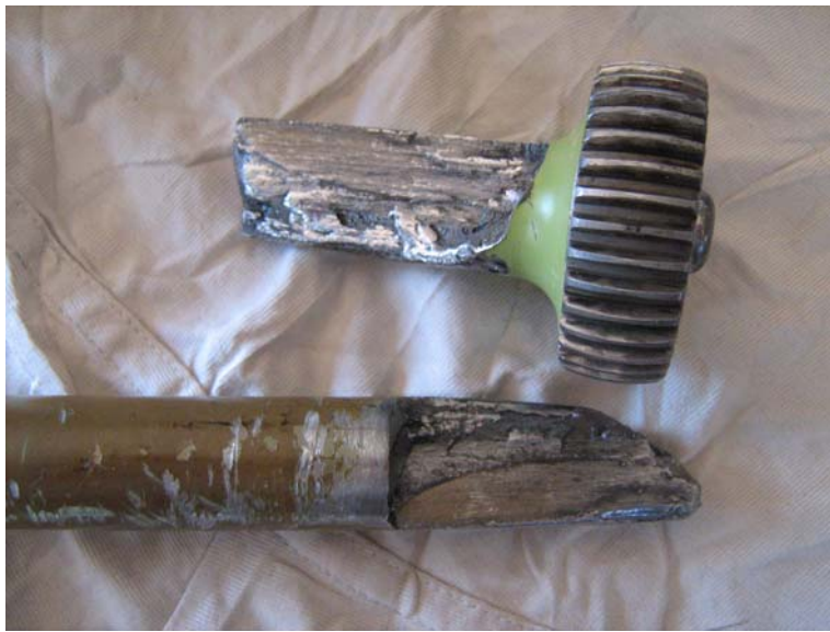
Figure 4. A view of the failed driveshaft after it was cleaned (grease removed).
