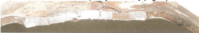
Photo 18: Clutch pulley frame fracture surfaces (digital)
