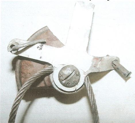
Photo 15: Fractured clutch pulley assemble (digital)
