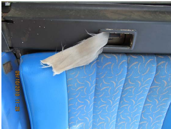
Figure 2. A view of the failed shoulder harness at the left seat (pilot side).
