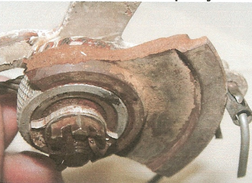
Photo 16: Fractured clutch pulley assemble (digital)
