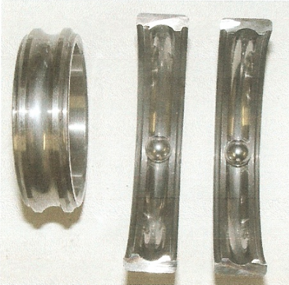
Photo 13: Lab opened bearing balls and raceway surfaces (digital)
