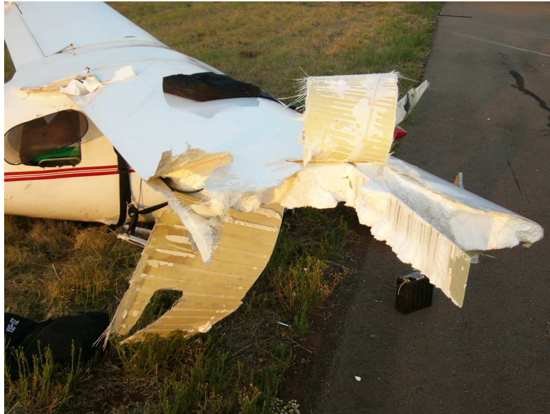
Figure 11. Damage caused to the right and aileron of ZU-BXA.
