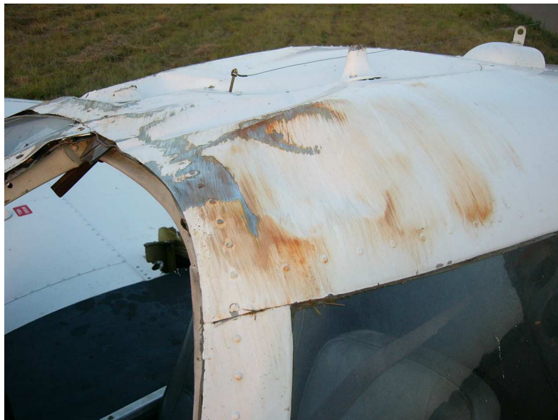
Figure 12. Abrasion and ground smear marks on the canopy of ZS-KIN.
