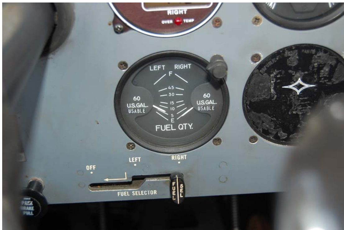
Figure 6. Position of the fuel tank selector immediately after the accident.
