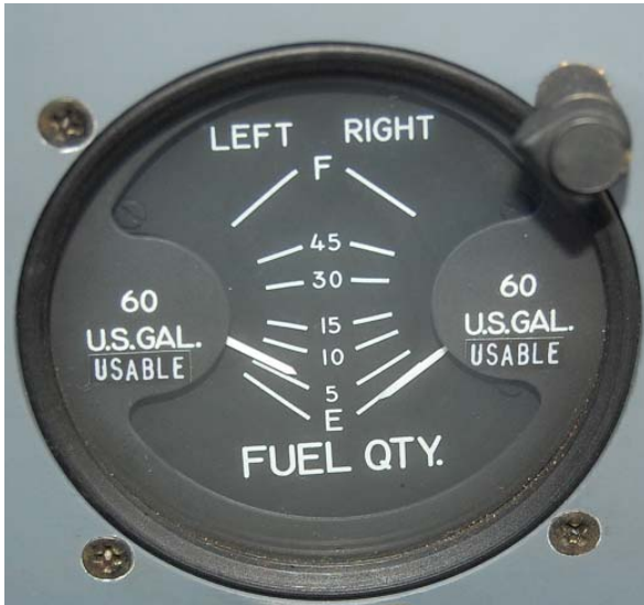
Figure 3. Readings in a nose-down attitude.
