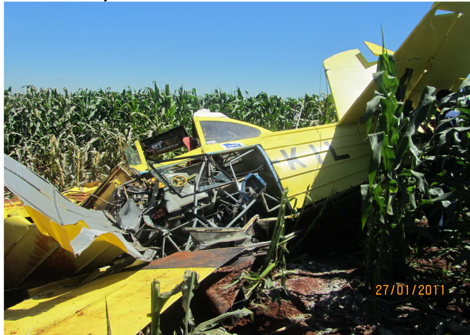
Photo 1: View of substantial damage caused to the aircraft fuselage, cockpit window frame and wings.
