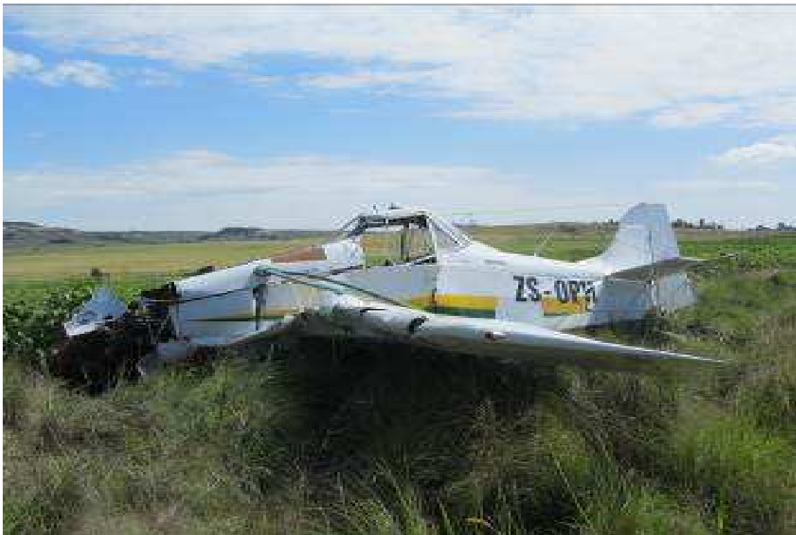
Figure 3: The damage to the left side of the aircraft.
