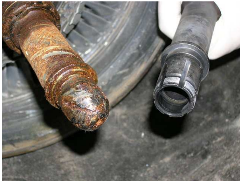
Photo No. 18 Power turbine shaft forward section compared to exemplar shaft.
