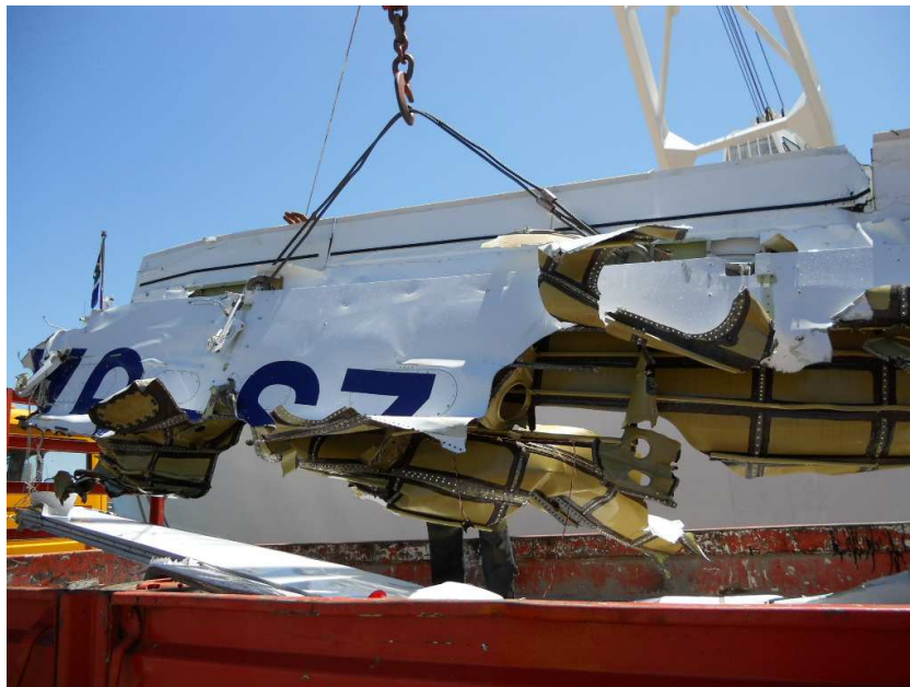
Figure 7: A view of the left wing that was recovered with a section of the flap attached.
