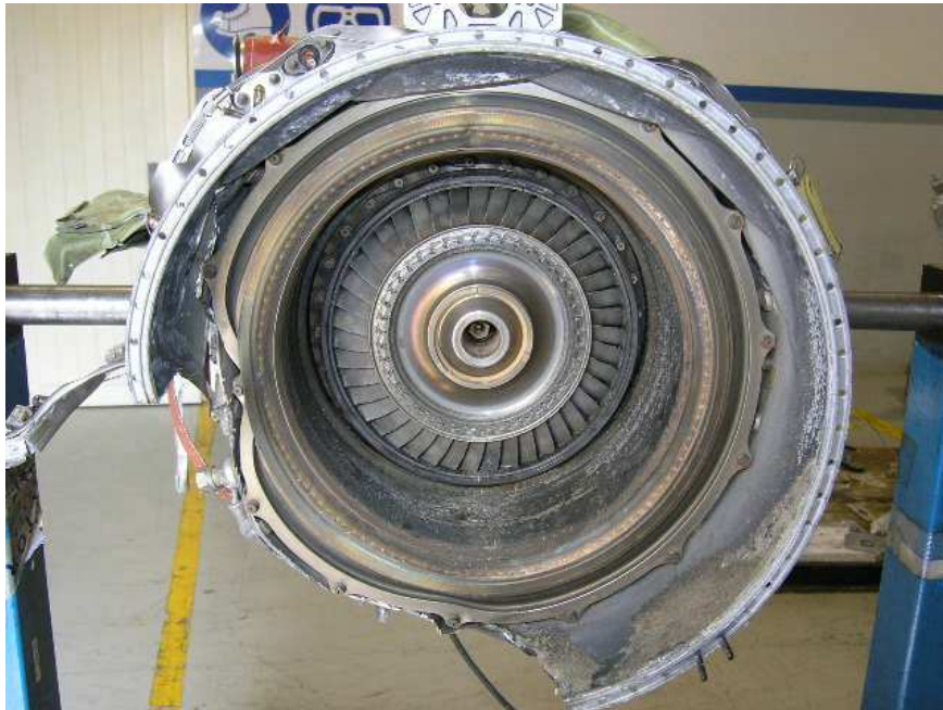
Photo No. 6 Combustion chamber liner and compressor turbine, in-situ.
