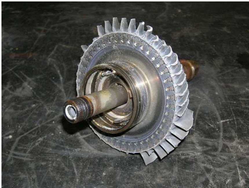
Photo No. 15 2nd stage power turbine and power turbine shaft, upstream side.
