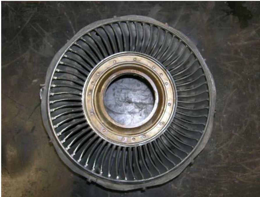
Photo No. 12 2nd stage power turbine vane ring, upstream side.
