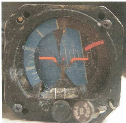
Photo 3: ZS-GAA Attitude Indicator, faceplate indication, as supplied (digital)
