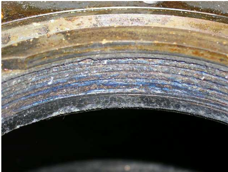
Photo No. 13 Interstage abradable airseal detail, approximate 9:00 position.
