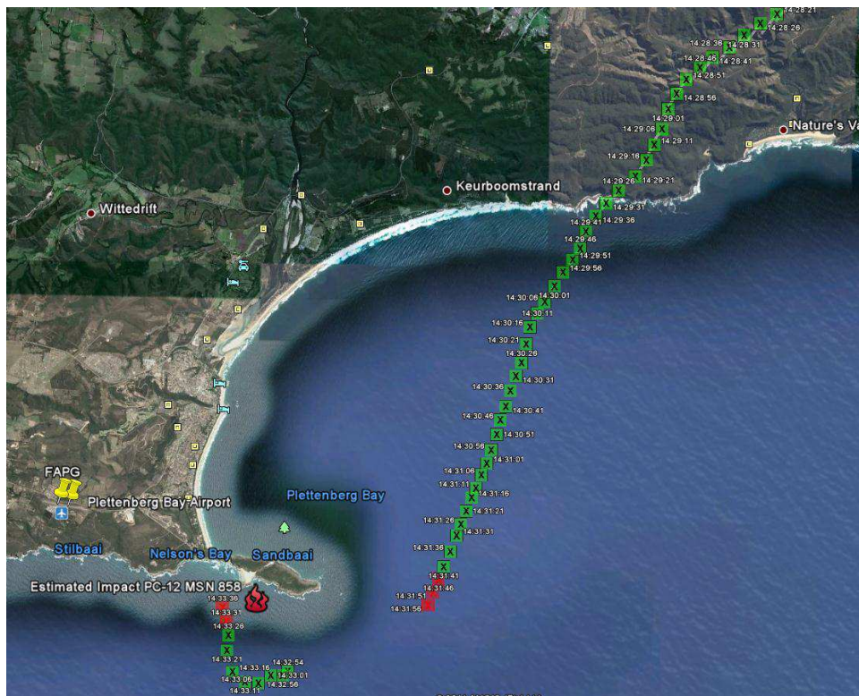
A clip of the radar footage reflecting the accident aircraft's approach path for an intended landing at FAPG.
