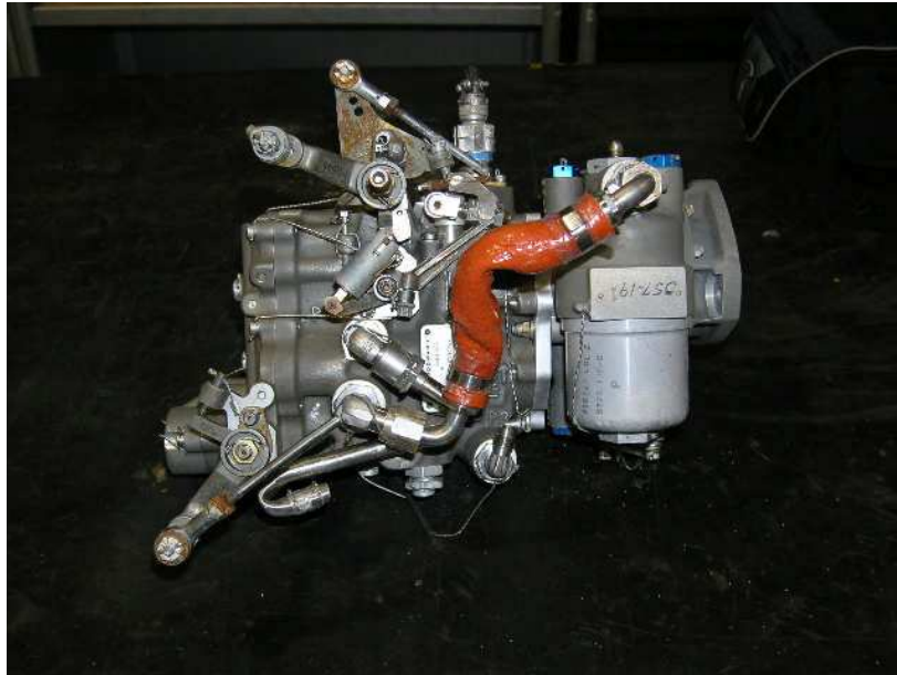
Photo No. 21 Fuel control unit and high pressure pump, right hand view
