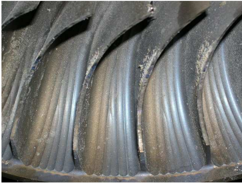
Photo No. 4 Centrifugal impeller detail.
