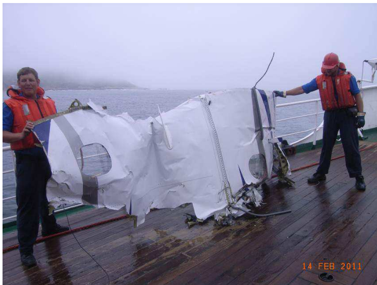
Figure 13. Top part of cargo area fuselage section.
