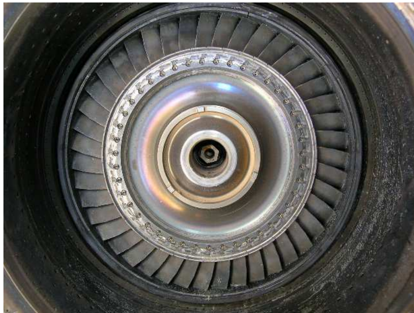
Photo No. 7 Compressor turbine, in-situ.
