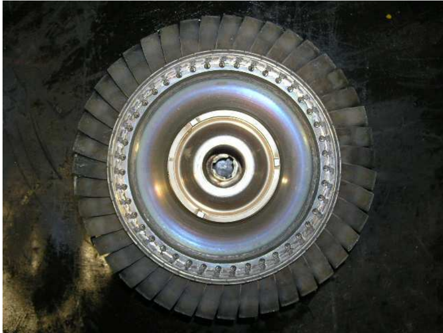
Photo No. 8 Compressor turbine, downstream side.
