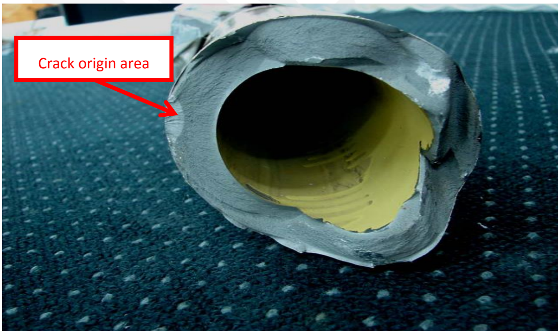
Photo 5. Fracture surface exhibited beach marks / striations originating from the surface of the inner radius of the bend.
