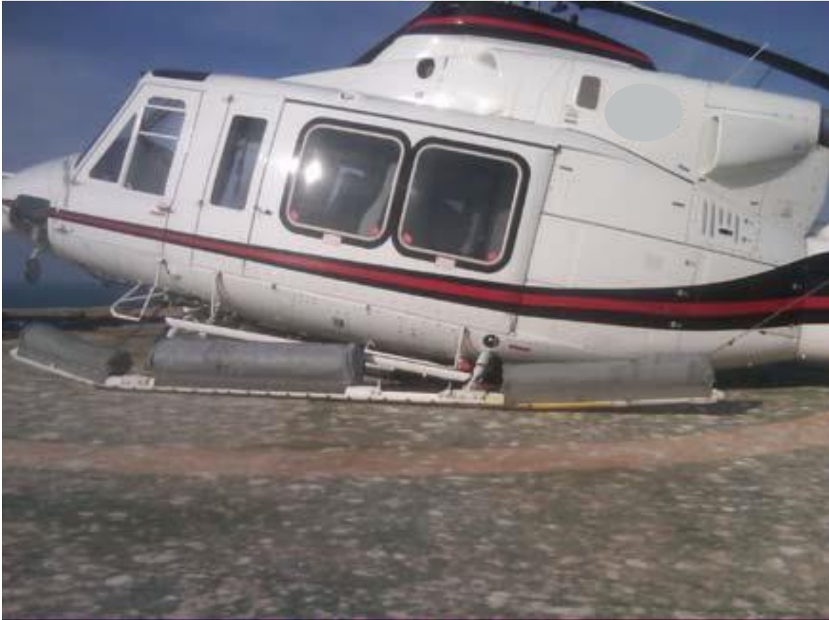
Photo 1. A6-FLV following aft crosstube failure
