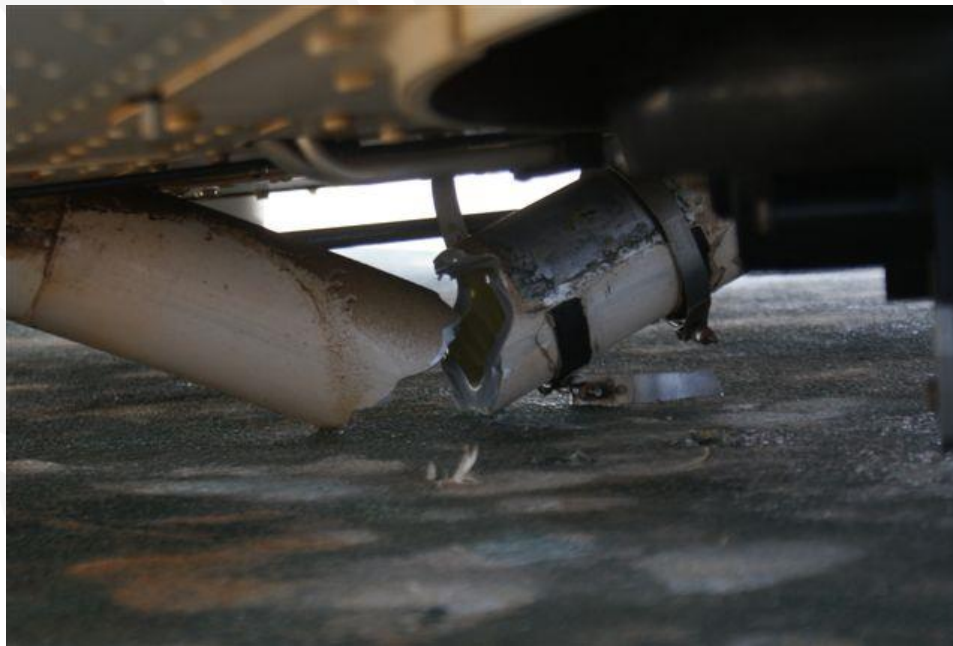
Photo 2. Failed Undercarriage Aft Crosstube A6-FLV (looking aft)
