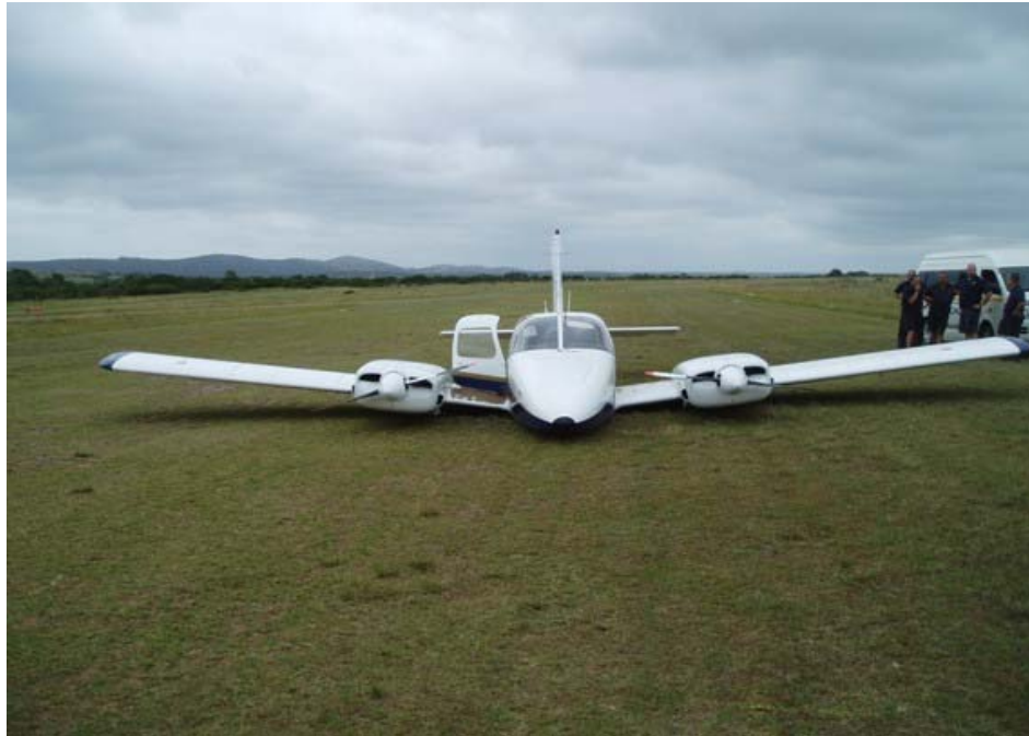
Figure 2. Front view of the aircraft after the wheels-up landing.
