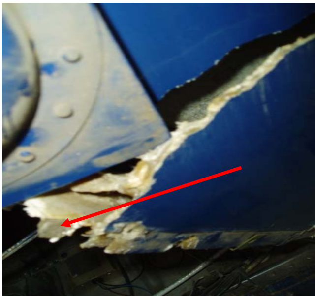
Figure 4. The discolouration indicates an earlier repair. A fibreglass spar which runs the length of this section of the nose cone is designed to provide some rigidity to the structure. This spar was fractured, enabling the entire nose to twist under the aerodynamic forces of the ram air entering the wheel bay when the doors were open. This twisting was sufficient to cause the side of the wheel bay to press against the undercarriage mechanism, thus preventing the nose wheel from extending.
