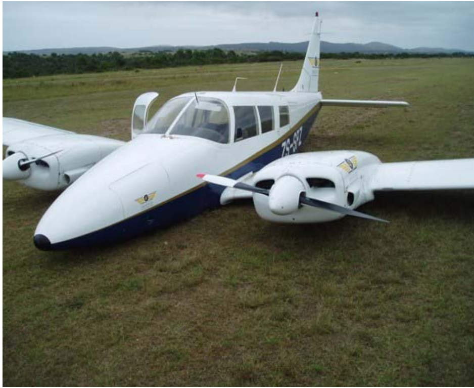
Figure 1. The aircraft after the wheels-up landing.
