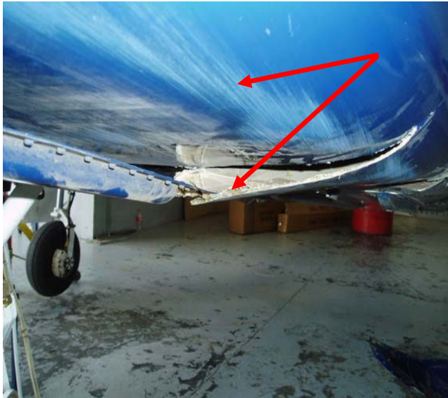
Figure 3. Tear in the fibreglass and scuffing on the lower surfaces.
