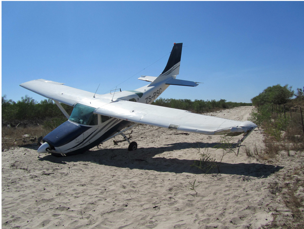
FIGURE 1 Damage to the wing tip and propeller
