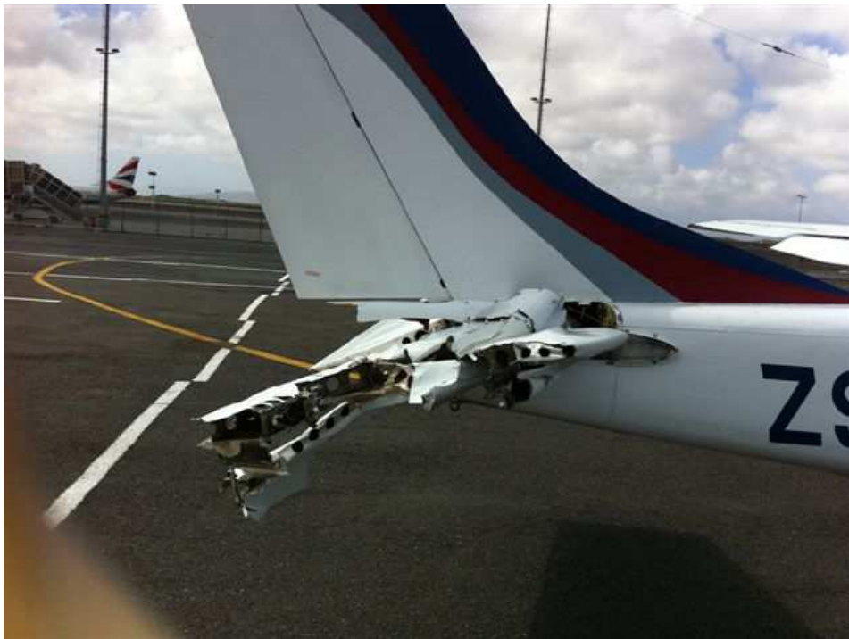
Figure 2: Side view of damaged elevator
