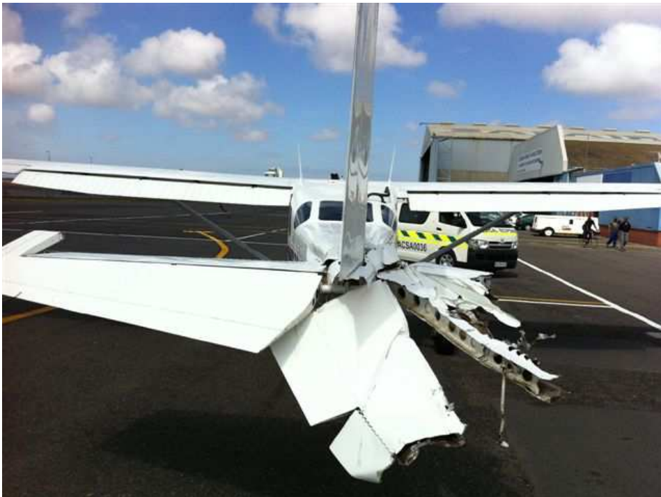
Figure 1: Shows the right hand vertical stabiliser severely damaged.
