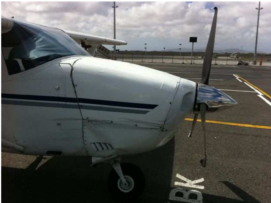
Figure 4: Side view of damaged propeller
