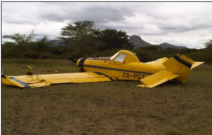
Figure 3, shows wreckage after the ground loop.
