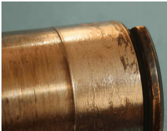
Figure 15 and 16, shows fretting damage on secondary rod big-end pin and loss of copper plating through wear on pin end.
