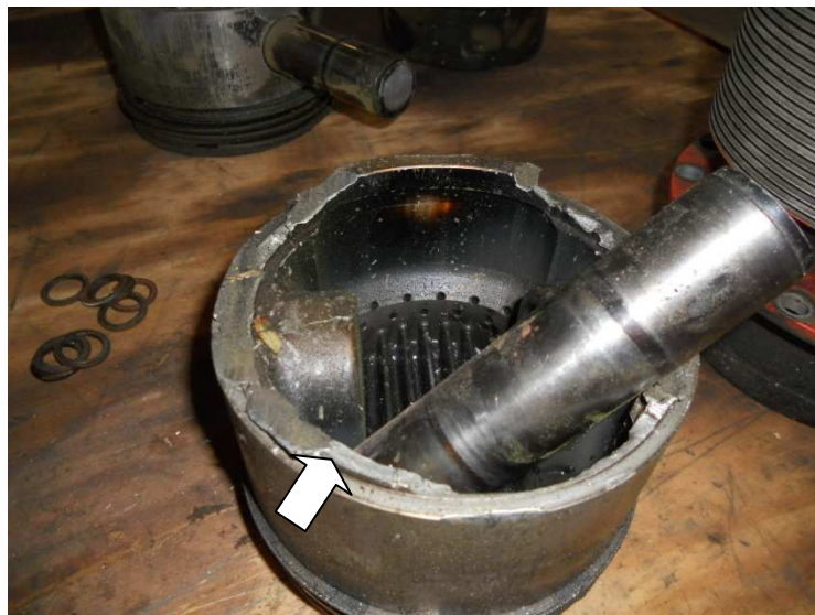
Figure 8, shows broken piston (#5 and #6) skirts.
