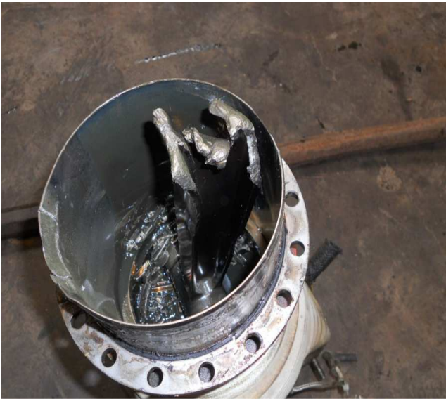
Figure 6 and 7, shows fractured master link rod on #5 & #6 cylinders.
