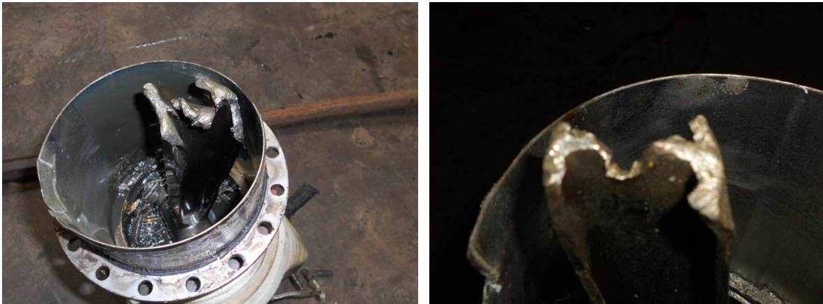
Figure 2 : Evidence of the piston rods failure.
