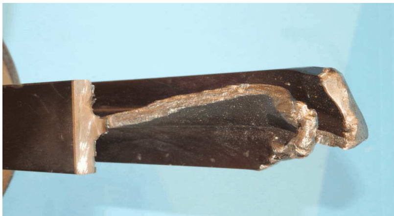
Figure 11, shows longitudinal and obliterated crack surface of master rod.
