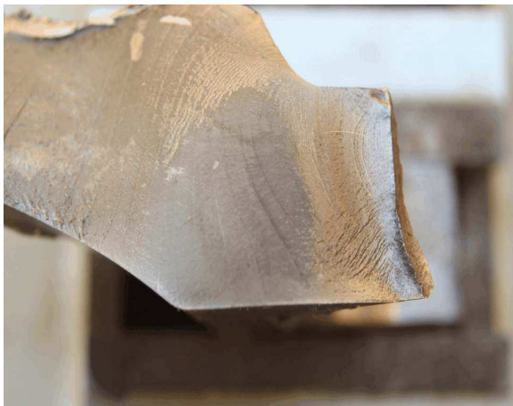
Figure 13 and 14, shows features typical of fatigue on the secondary crack and fretting corrosion deposits and scoring on secondary rod big-end hole on master rod.
