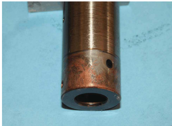
Figure 15 and 16, shows fretting damage on secondary rod big-end pin and loss of copper plating through wear on pin end.
