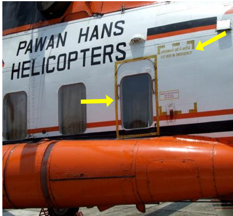
Photo : 17 Emergency Starboard Escape(Forward) and Cut Away
