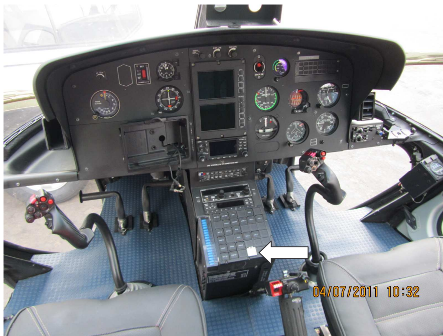
Figure 5. Position of the “ACCU TST” switch on the systems control panel.
