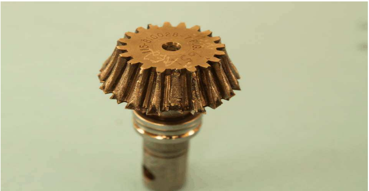
Figure 2 showing the extensive wear of teeth and missing tooth on the small drive gear.
