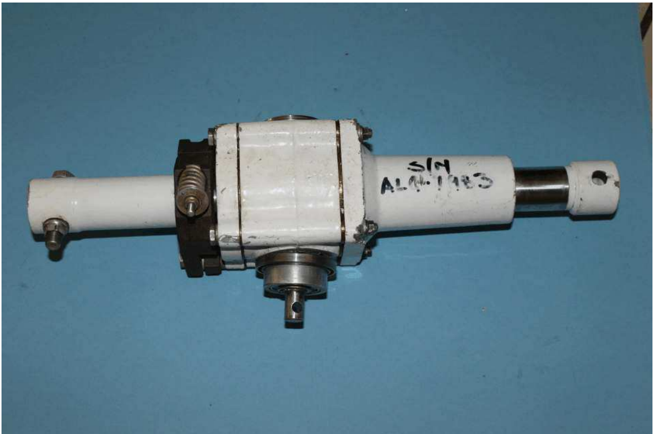
Figure 2 showing the right hand main landing gear actuator before disassembly
