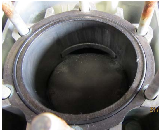
Figure 3, shows the piston that seized.
