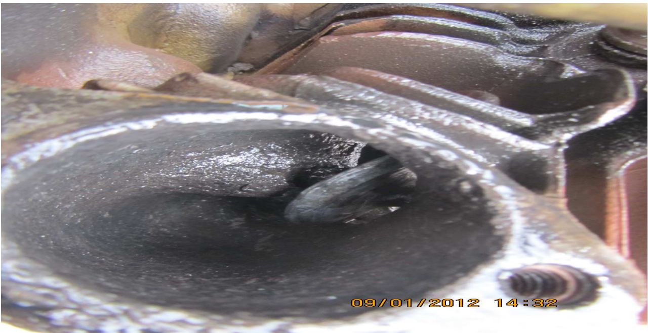
Figure 3: showing the exhaust valve head through the manifold port.
