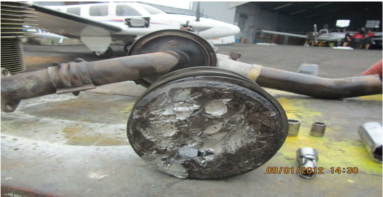
Figure 4: showing damage caused to the no.2 cylinder piston
