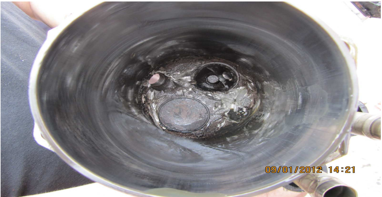
Figure 2: showing damage caused in the no. 2 cylinder chamber.
