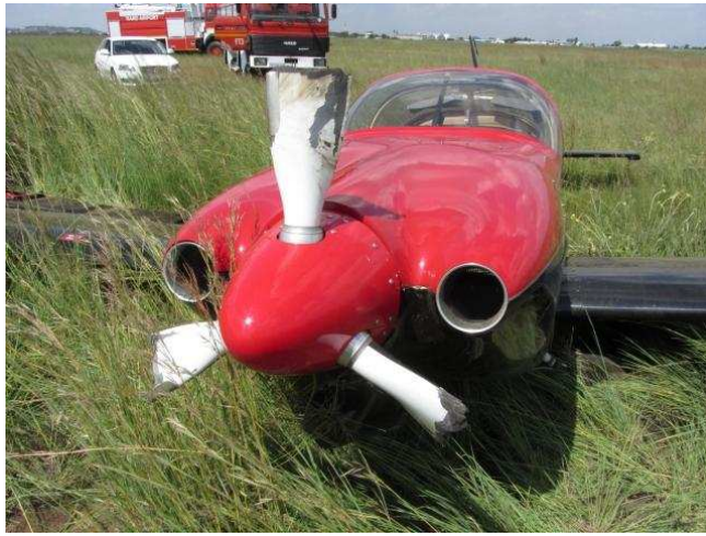
Fig.1 – Damage to the propeller
