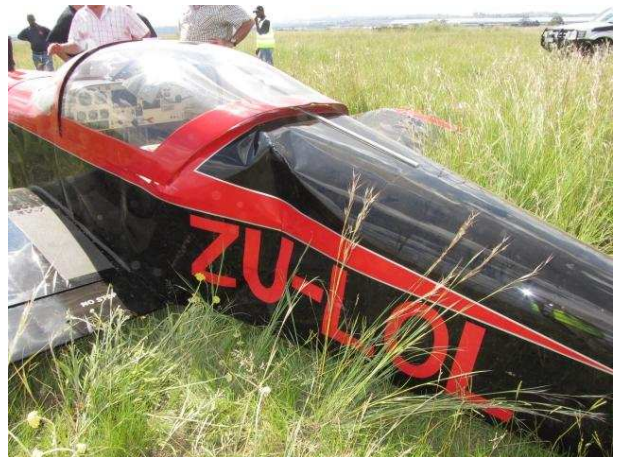
Fig. 3 – Damage to fuselage
