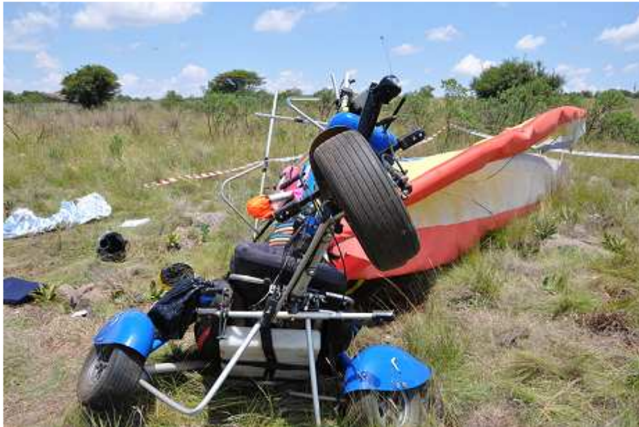
Figure 5, shows the damage caused to the airframe structure.
