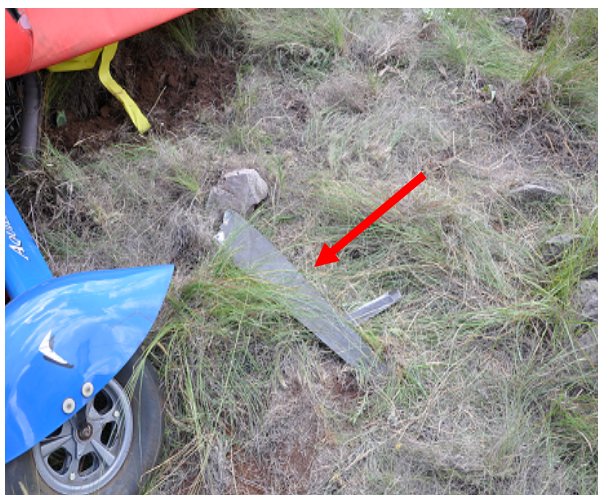
Figure 5 and 6, shows the damage caused to the propeller during the impact sequence.
