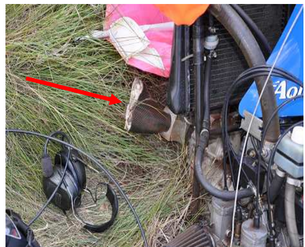
Figure 5 and 6, shows the damage caused to the propeller during the impact sequence.
