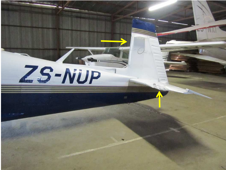
Figure 1, showing damage to the horizontal and vertical stabiliser.
