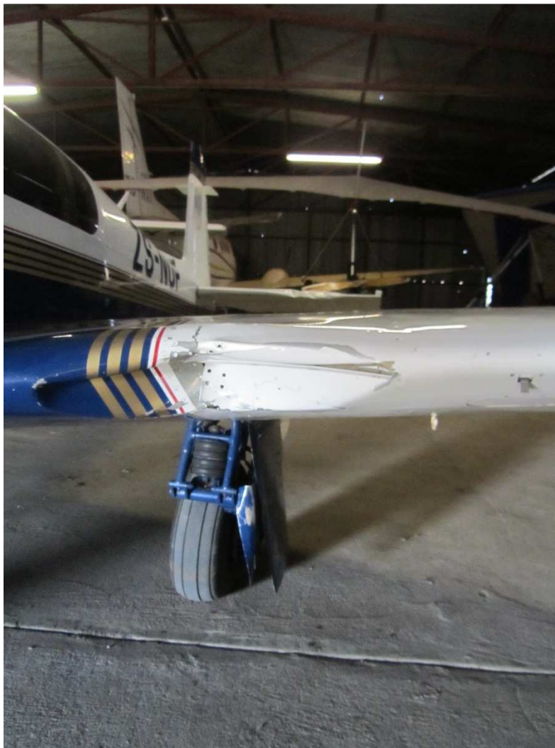
Figure 2, showing damage to the port-side wing.
