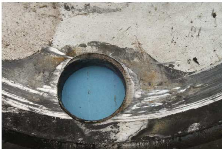
Figure 5. Burring of bolt holes on disk.
