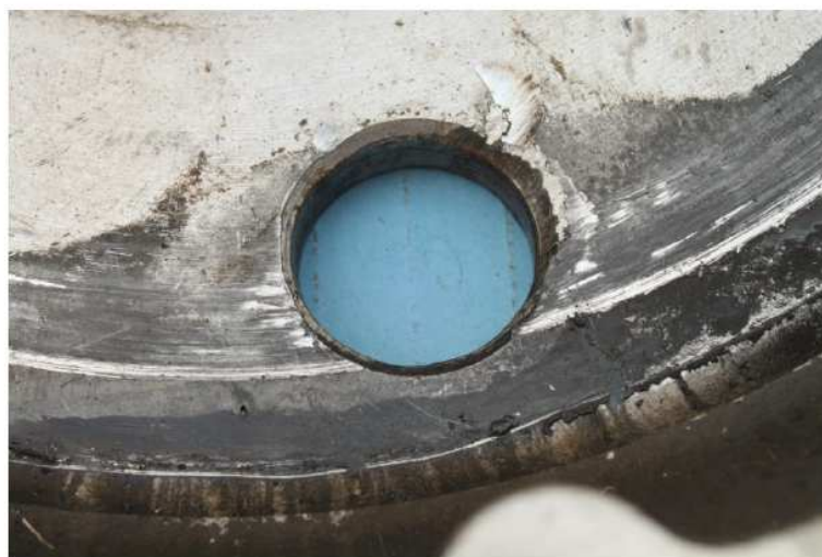
Figure 4. Burring of bolt holes on disk.
