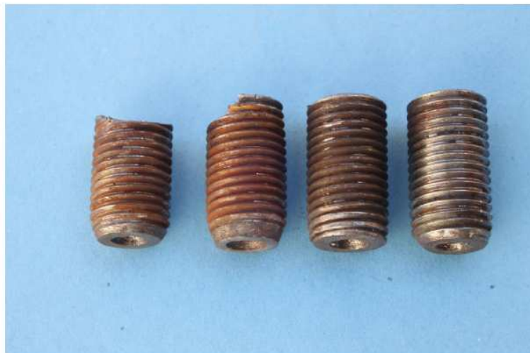
Figure 7. Corrosion observed on the threads after removal from the nuts.
