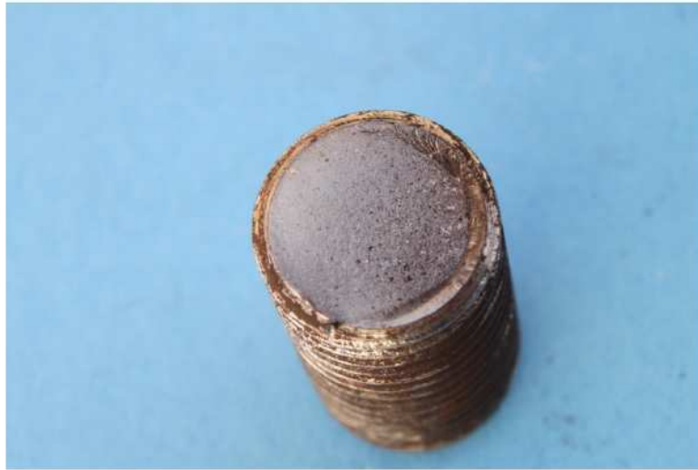
Figure 9. Apparent ratchet marks observed on another fastener indicating early stages of fatigue.
