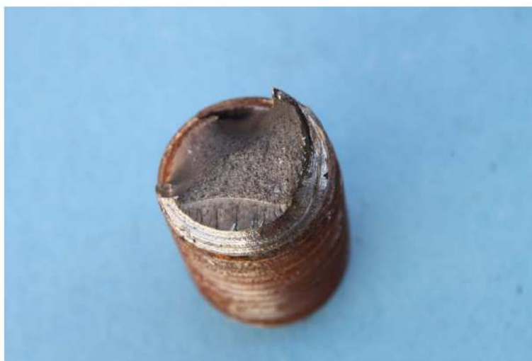
Figure 8. Characteristic features of fatigue observed on one fracture surface.
