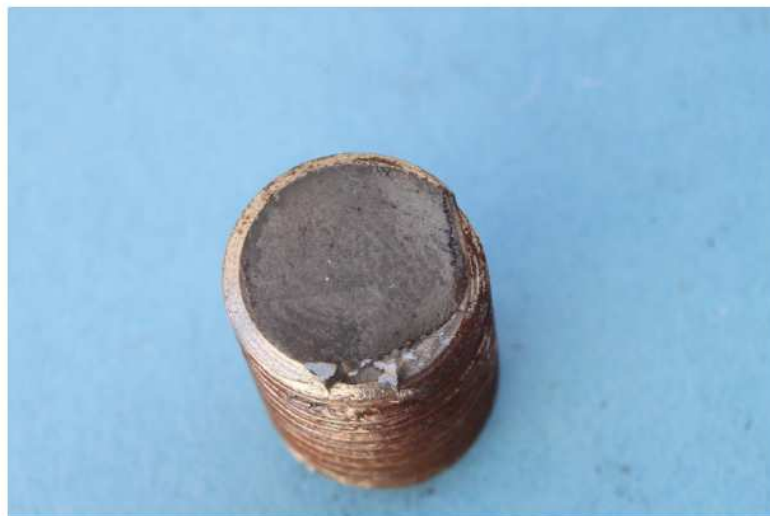
Figure 10. Apparent ratchet marks observed on another fastener indicating early stages of fatigue.
