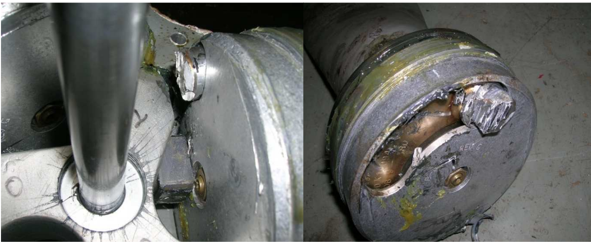
Figure 8 and 9: Evidence of damage on the blades inside the hub.
