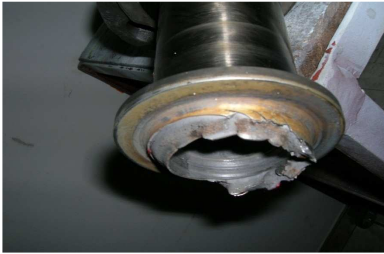
Figure 11: Evidence of damage on the crank shaft.
