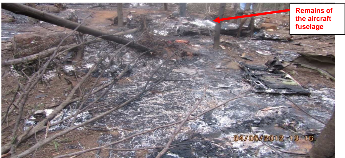
Figure 2: Aircraft wreckage, showing the extensive fire damage.
