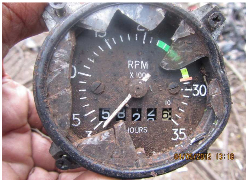
Figure 4: View of the aircraft tachometer as found at the accident site.
