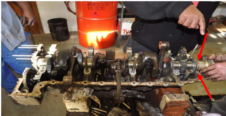
Figure 10: View of the crank shaft and severed flange.
