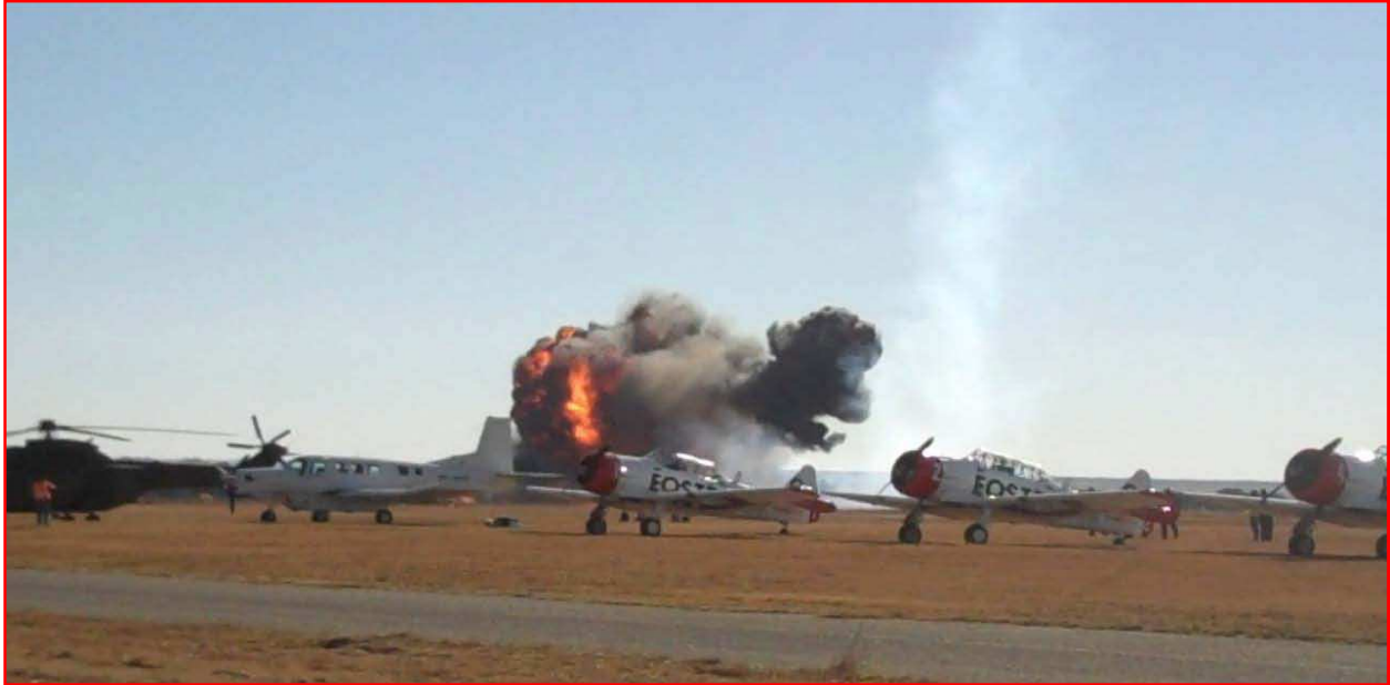
Figure 8: The aircraft exploded and a post impact fire erupted during the ground impact
