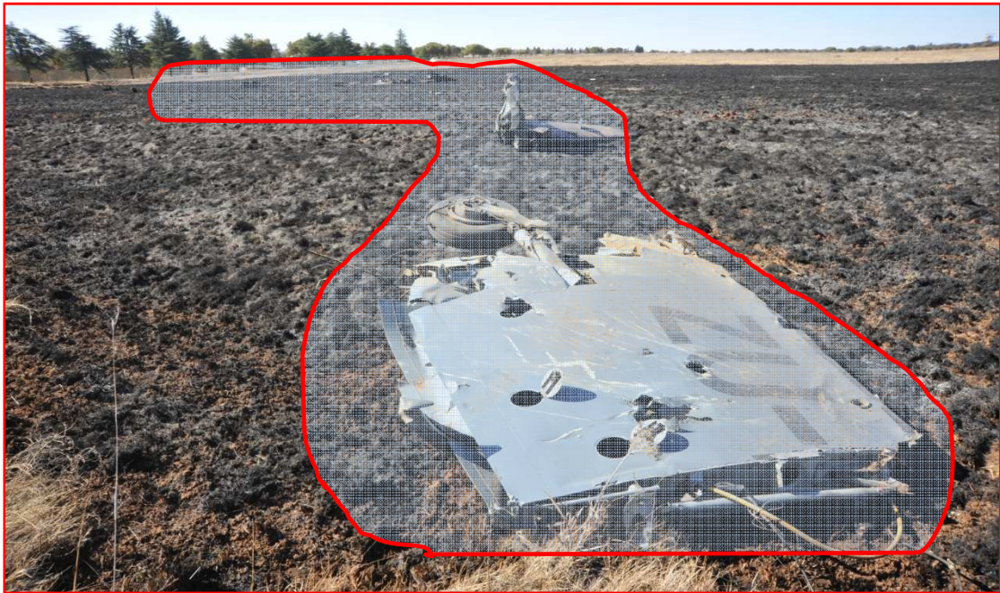
Figure 2: Wreckage pieces were spread over a distance of approximately 300m
