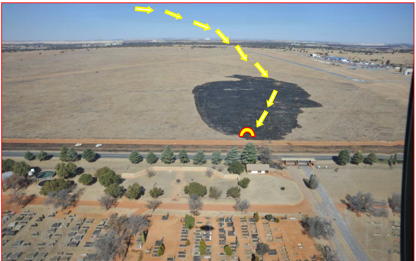
Figure 7: Shows a view of the approximate flight path followed by the aircraft with the position of the forward cockpit as indicated.
