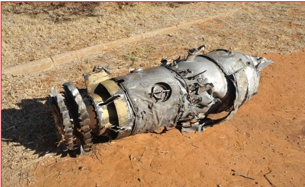
Figure 1: The main core of the turbine engine that separated from the A/C on impact
