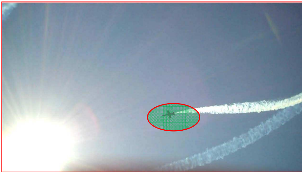
Figure 15: The accident aircraft is now inverted. Note the vertical fin facing downward
