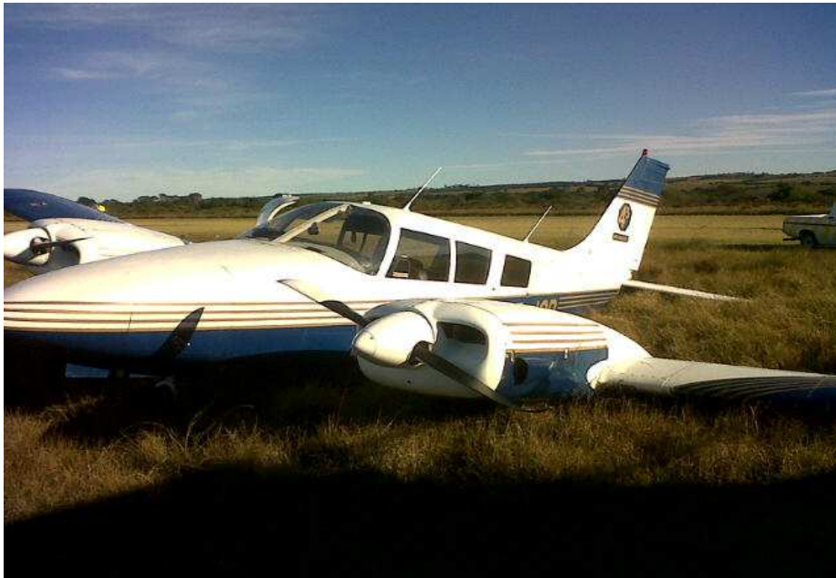
Figure 1, shows aircraft with left main landing gear collapsed.
