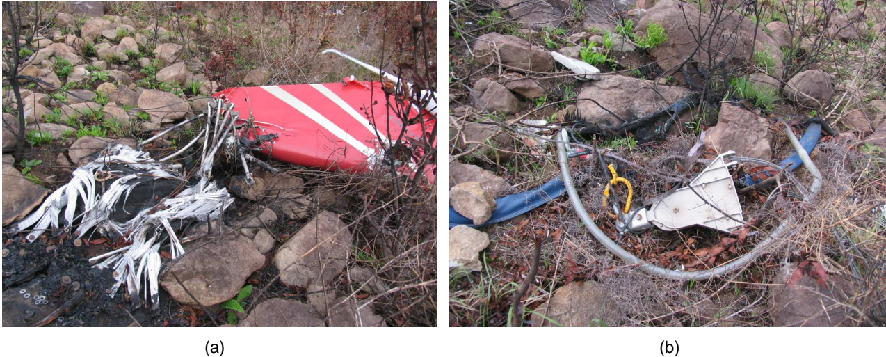
Figure 9. Burnt out bambi bucket next to the tail boom pylon (a) and cargo sling cabling with bambi bucket hook (b).
