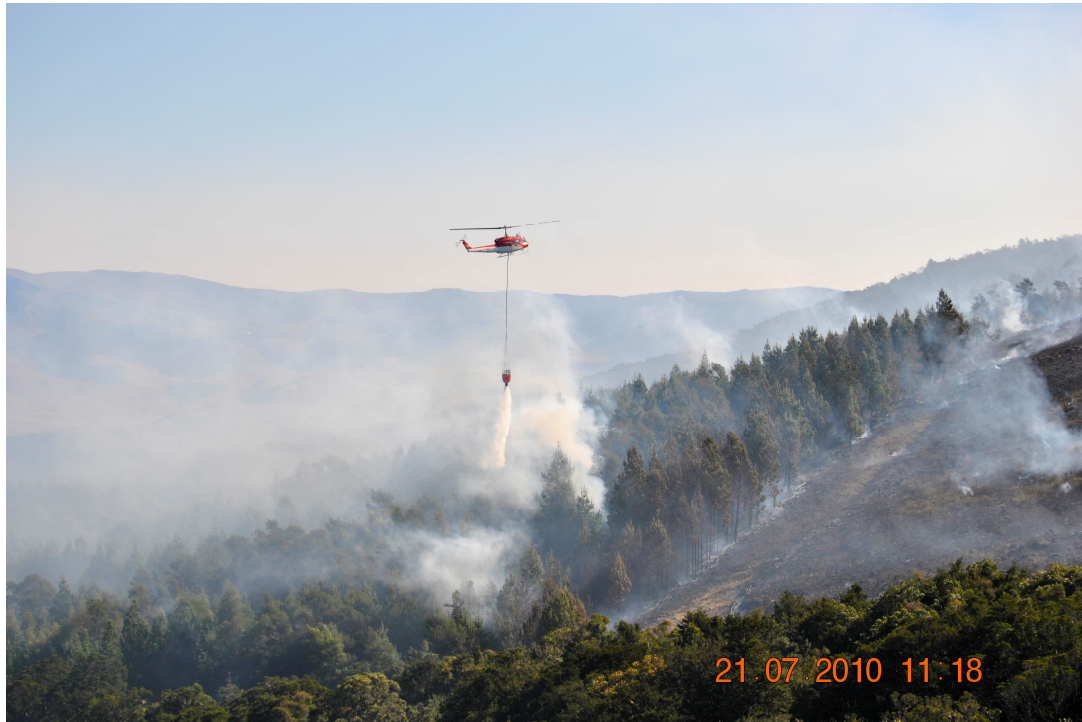
Figure 5. A Garlick UH-1H helicopter engaged in a fire fighting operation slinging a bambi bucket.
