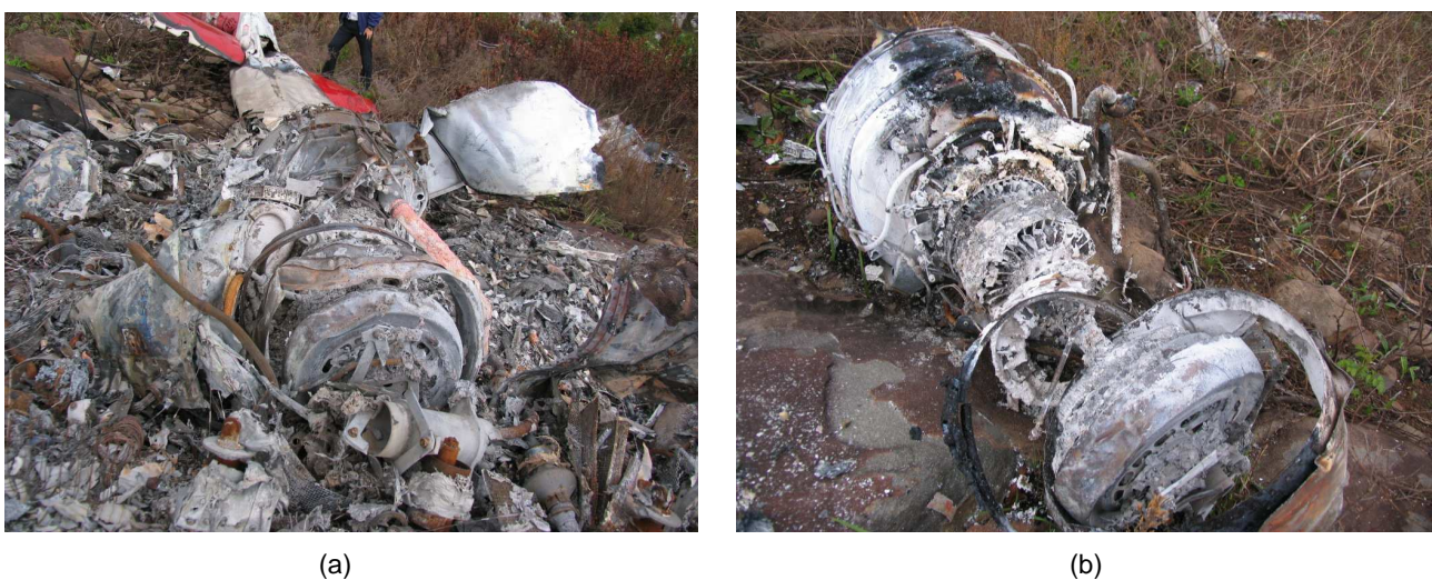
Figure 10. A view of the engine before (a) and after it was removed from the burnt out sheet metal structure (b).
