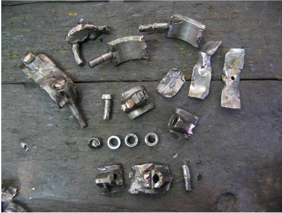
Figure 5. The photo shows some of the debris that was recovered from the sump of the engine.
