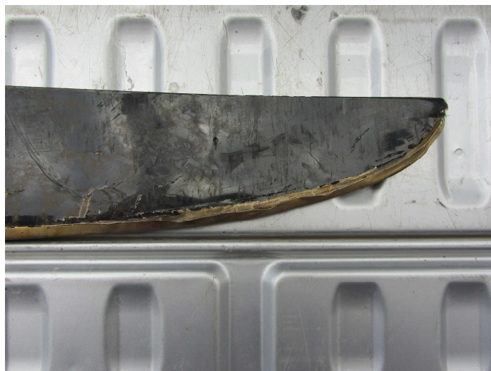
Figure 9 A third propeller blade found underneath the wreckage without any damage indicating rotation-associated with normal engine operation (to sustain flight).
