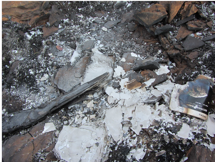
Figure 8 A second propeller found close to the wreckage without any sign of damage caused by rotation.
