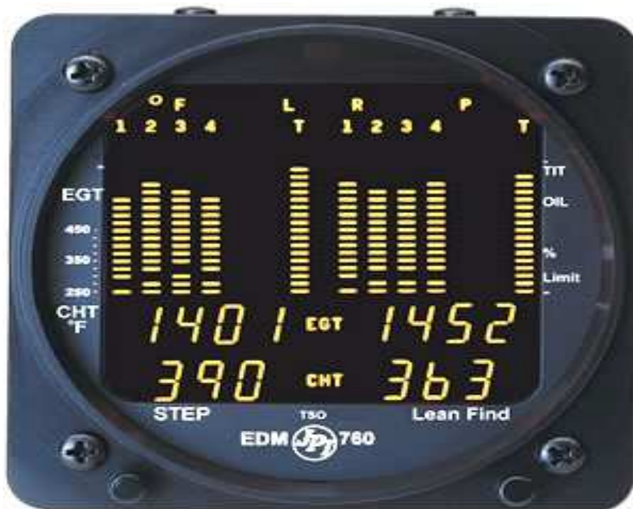
Figure 6: View of a twin six cylinder EDM-760 monitor.
