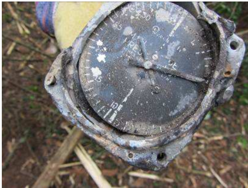
Figure 13. A photo of the manifold pressure and fuel flow gauge that was recovered on site.
