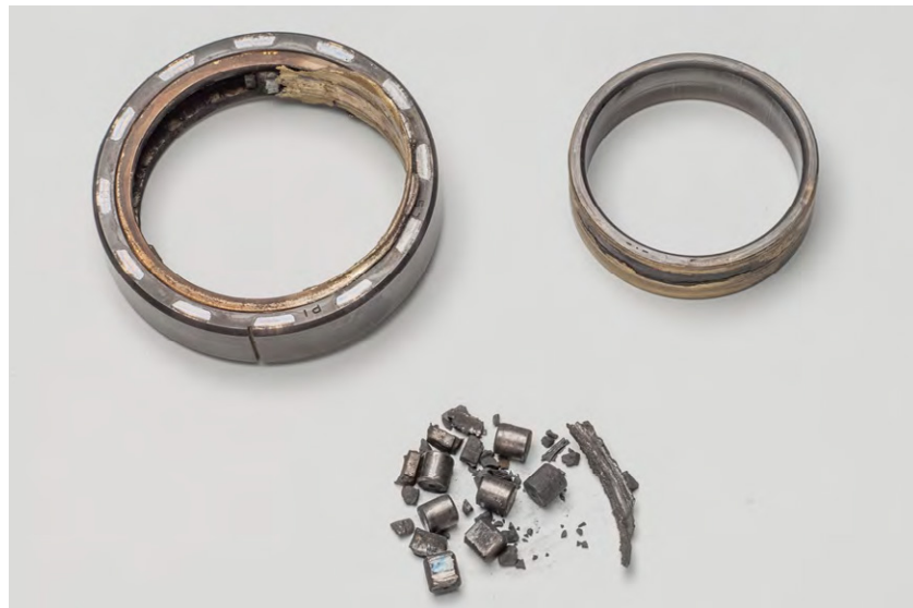
Fig. 1 Overview of the failed bearing components
