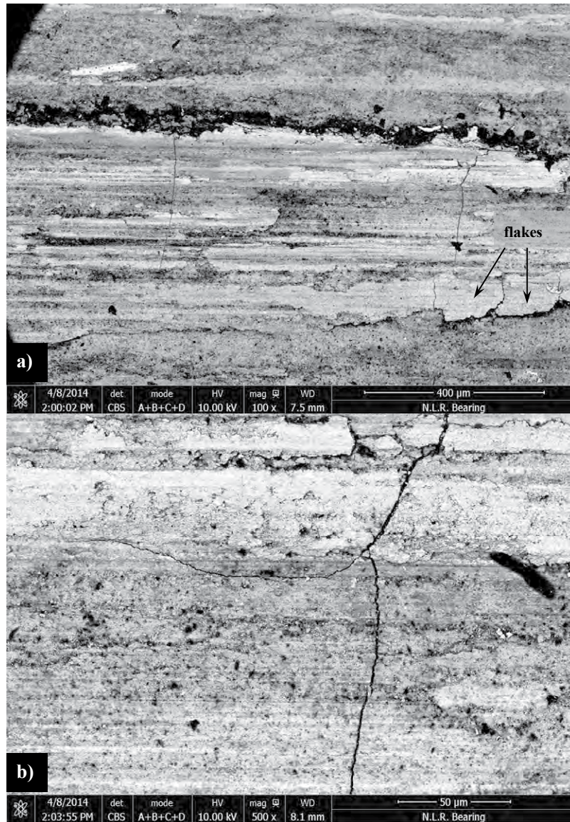
Fig. 8 SEM image of the black inner raceway surface at a) 100x and b) 500x magnification
