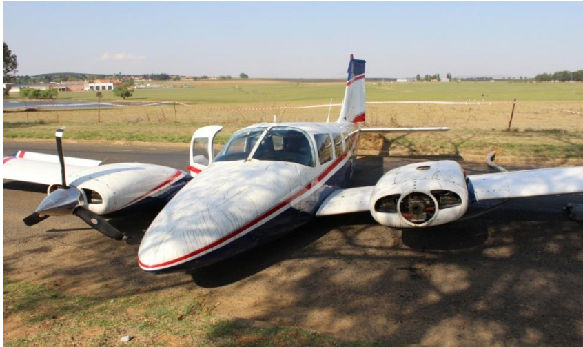
Figure 3: Damage to the left and right hand propellers
