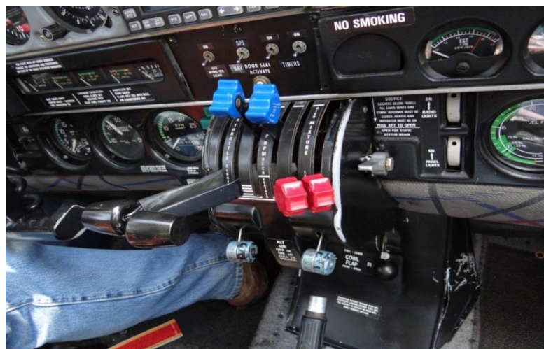
Figure 5: Propeller pitch levers on full forward
