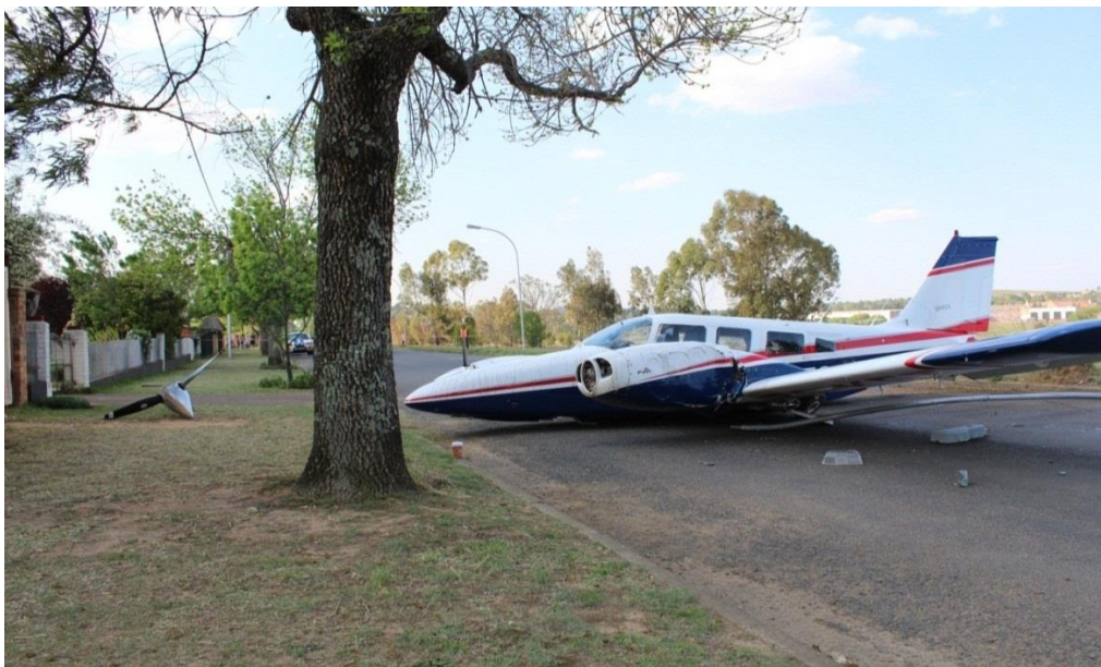
FIGURE 1: ZS-KFT ON ROAD WITH L/H ENGINE PROP FAILED ON IMPACT WITH STREET POLE LIGHT
