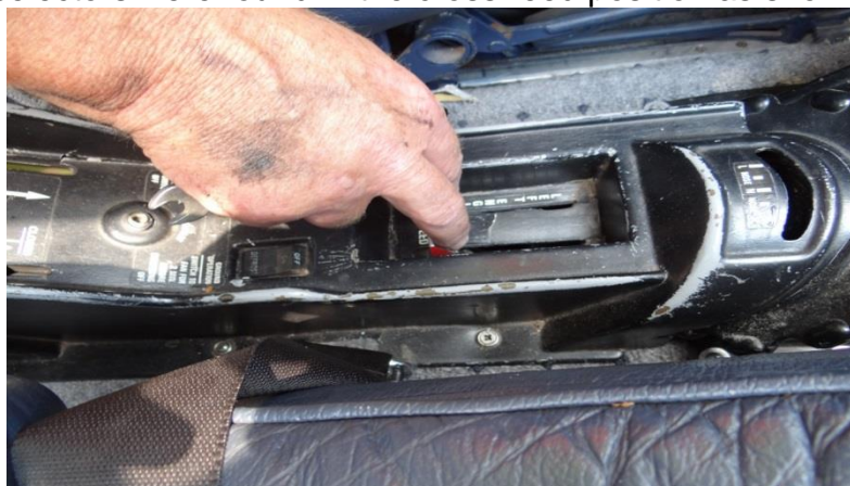
Figure 6: shows both fuel selectors on the cross-feed position
