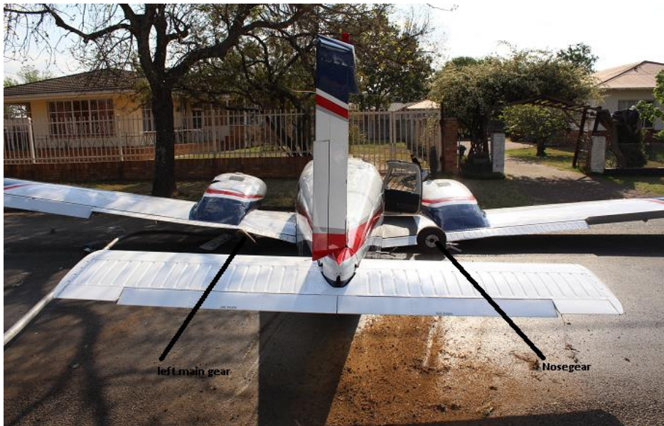
Figure 4: left main landing gear & nose landing gear damage
