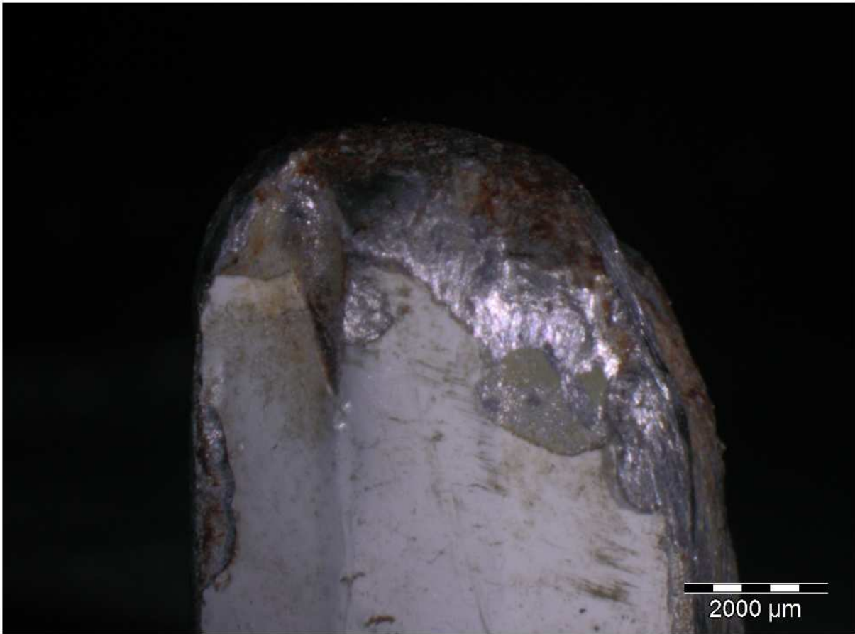
Figure 5: Side view of dull fracture end, showing additional mechanical damage to the side walls.
