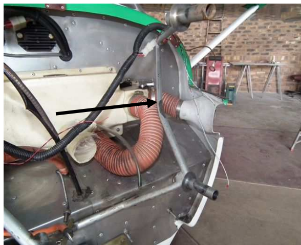
Figure 4: Shows the engine cradle bent.
