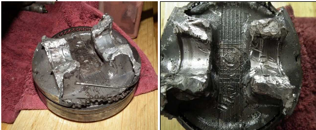
Figure 6 and 7: Shows damage caused No 2 engine piston.
