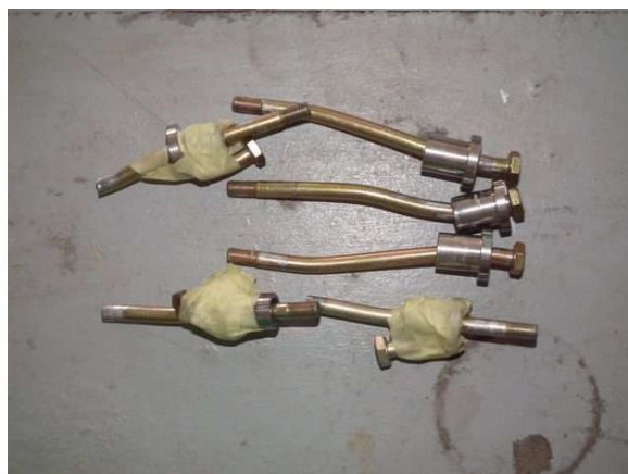
Figure No 2 & No 3: Shows damage to the propeller and the bolts bent during sudden stoppage of the engine in flight.
